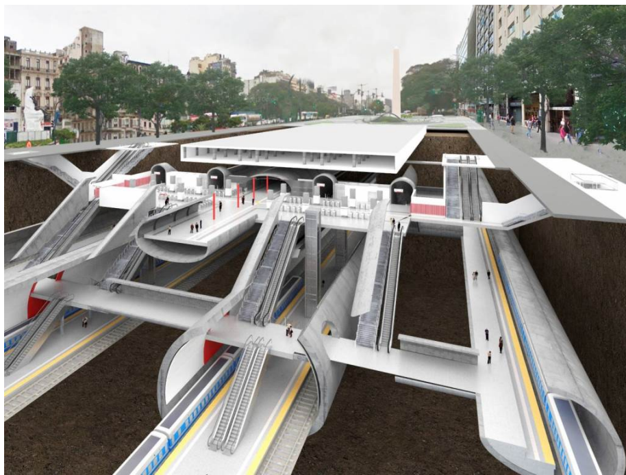
Figure 28: RER: Computerized image of a proposed subterranean transfer station under the obelisk, in downtown Buenos Aires. Source: Railway Gazette 2018. Downloaded from http://www.railwaygazette.com/news/news/cs-america/single-view/view/buenos-aires-rer-to-be-built-through-a-ppp-1.html?word_list%5b%5d=argentina&no_cache=1 in March 2018.
