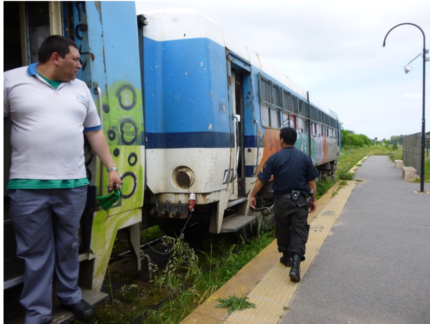
Figure 17: The light train colloquially known as Pitufo, “Smurf,” by railroad workers, serving Victoria - Capilla del Señor. It has been nicknamed “The Cocktail Shaker” by activists due to the jerks and jolts caused by poorly maintained tracks. Notice that the tracks are barely visible due to weeds. Photo by author.
