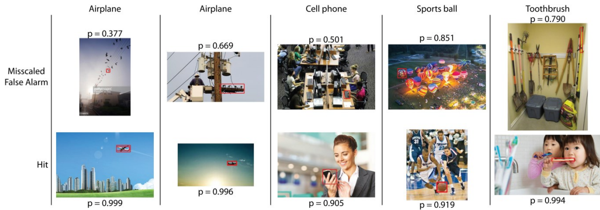
Figure 35: Top row – instances where the object detector mis-classifies with high probability an object category of inconsistent scale with the actual object region. Bottom row – correct classifications of the same object categories for comparison.
