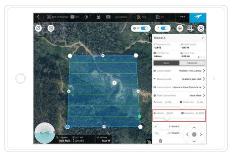
Navigate to Advanced, and select the overlap on both front and side overlap. This is 80% for high-altitude flights and 85% for low-altitude flights.
