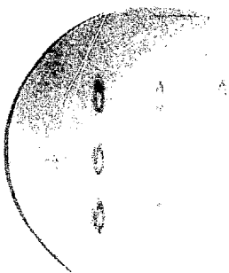
Nine Beam Witness Plate, 1" after end of MEQALAC.
