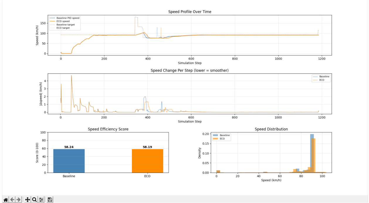
Fig. 6. Speed efficiency analysis for the platoon joining scenario, showing the four-panel output of analyze_speed.py .
