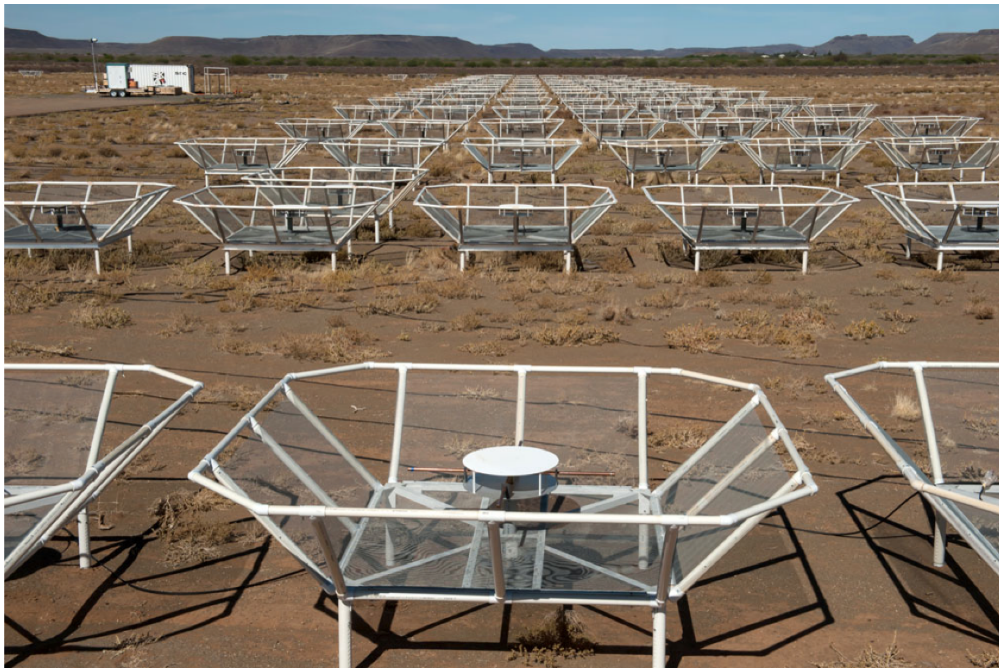
Figure 1.3: The Donald C. Backer Precision Array for Probing the Epoch of Reionization (PAPER) in its 128 antenna redundant configuration in September 2013. Located in the Karoo Desert in South Africa on the SKA Radio Reserve, PAPER arranged its antennas in a grid configuration to boost sensitivity in the Power Spectrum due to its limited collecting area.
