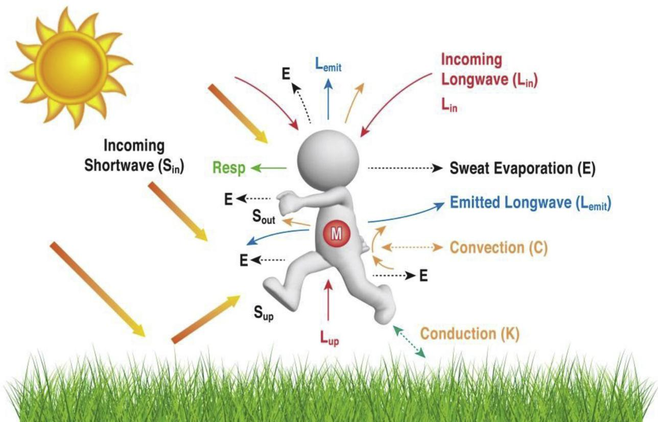
**Fig. 2 – Heat exchange between the environment and human body in an outdoor environment. In normal conditions, a human's energy balance will increase due to metabolic heat generation ( $M$ ) and radiation in the form of shortwave ( $S_{in}$  and  $S_{up}$ ) and longwave ( $L_{in}$  and  $L_{up}$ ) from the sky and ground. A human will normally lose heat through convection ( $C$ ), evaporation ( $E$ ), emitted longwave radiation ( $L_{emit}$ ) and respiration ( $Resp$ ).**
