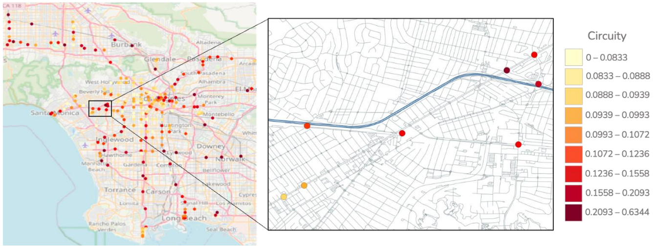
Figure 9: Street-network circuitry at major transit stations and stops. The measure indicates the log ratio of network distance to straight-line distance from the stop/station to other nodes within 500m. The stops/stations indicated consist of rail and Bus Rapid Transit stations, together with major bus stops as defined by Los Angeles Metro. The right panel shows stops/stations located in the Palms neighborhood of Los Angeles and in Culver City, with the freeway (I-10) in blue. The impact of the freeway in increasing circuitry is most evident at the bus stops in the upper right of the figure.
