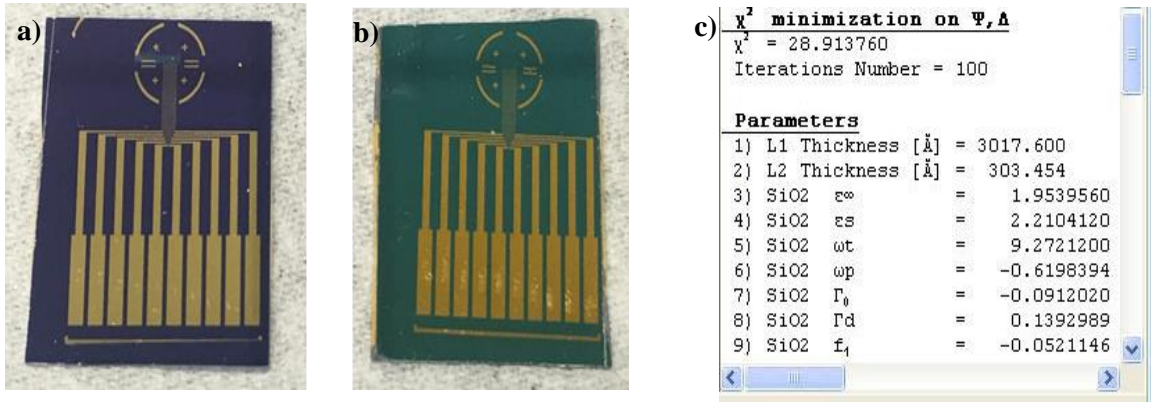
Figure C6. Optical image of the sensor (a) before and (b) after Al 2 O 3 deposition (c) L1: SiO 2 and L2: Al 2 O 3 thickness measured by ellipsometer.
