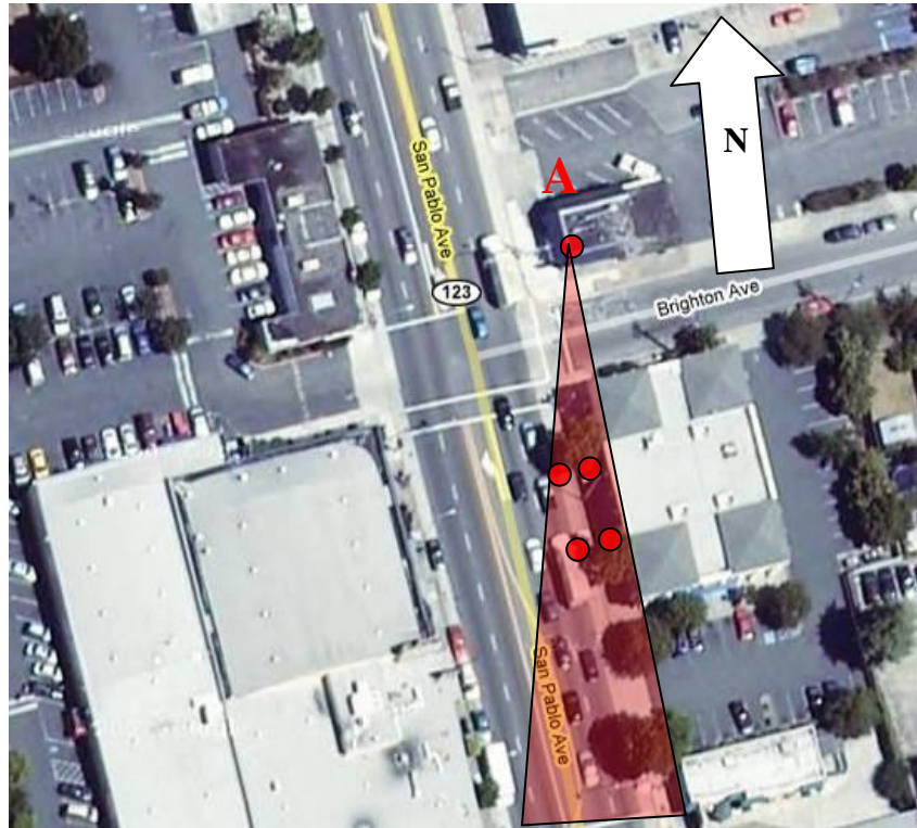
Figure 58, Sensor Placement near the intersection of Brighton and San Pablo Ave (Radar Antenna is placed at Location A, which is near the northeastern corner of the intersection, facing a southerly direction)
