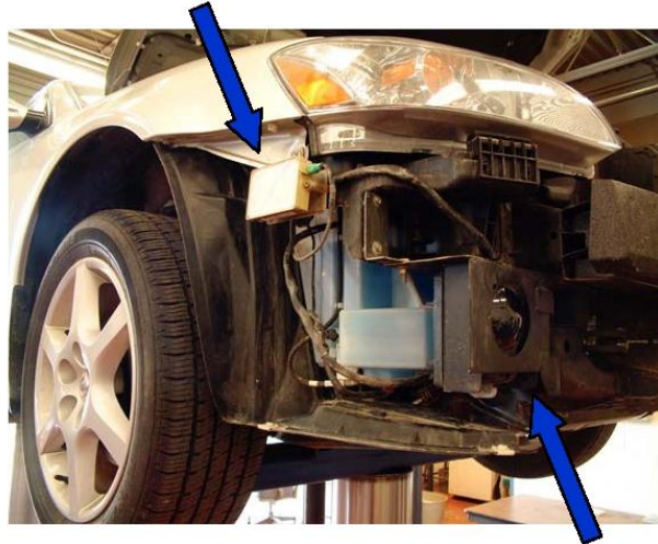
Figure A.3. Physical installation of the forward and side radars. (Reproduced from [7])
