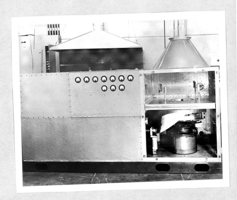
Fig. 9. An interior view of the final amplifier of the 90-inch cyclotron showing the filament transformer, grid capacitor, and ground plane. (The A2332 is removed.)
