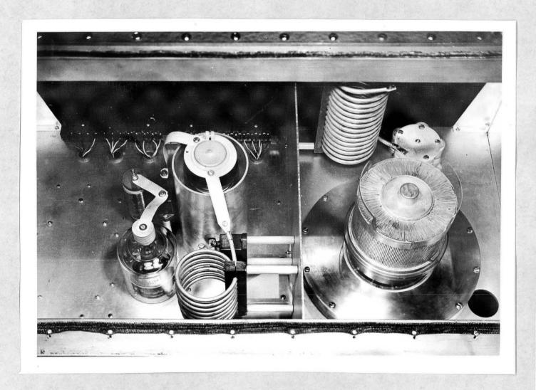
Fig. 11. The Driver Amplifier of the 90-inch Cyclotron. The tubes shown are the 4-250 and the 6166.
