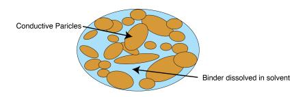
Figure 1.9: Conductive inks are made of discrete micro- or nano- particles of the conductive material, dispersed in a solution of solvent, polymer binder, and additives.
