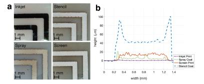
Figure 4.5: a) Microscope images of the top-left corner of the antenna show surface and edge roughness of patterns made with inkjet, stencil, screen, and spray printing (in a clockwise direction). b) Profiles of traces printed with the same four techniques. The vertical axis shows the trace height, while the horizontal axis shows the traces' transverse direction. The colors indicate different printing techniques.
