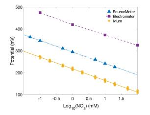
Figure 5.12: Measurement tools with sufficient  $Z_{in}$  allow readings of sensors with high sensitivity, but different  $E_0$  depending on the tool.
