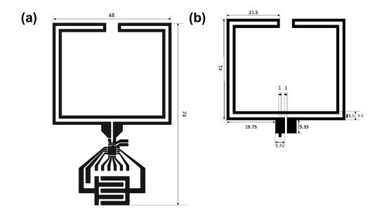
Figure 4.4: Dimensions of a printed folded dipole antenna. a) Complete RFID tag including the antenna, traces for mounting the IC and matching inductor, and printed capacitive touch sensor. b) The antenna alone used for S11 and radiation pattern measurements.
