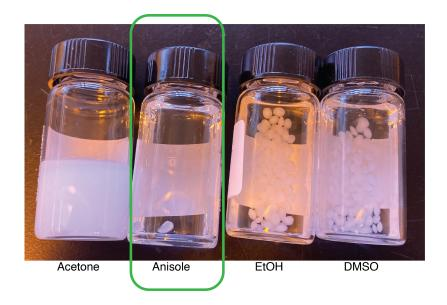
Figure 2.9: 1:8 by weight PCL in acetone solidifies at room temperature. 1:8 PCL in anisole dissolves well. 1:8 PCL in Ethyl Alcohol and and 1:8 PCL in DMSO does not dissolve.
