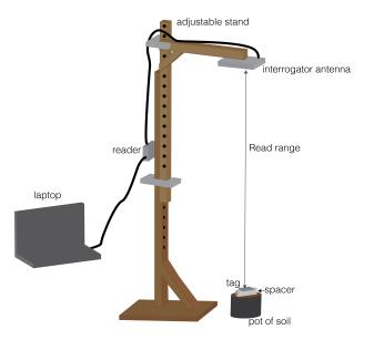
Figure 6.8: Read range measurement set up.
