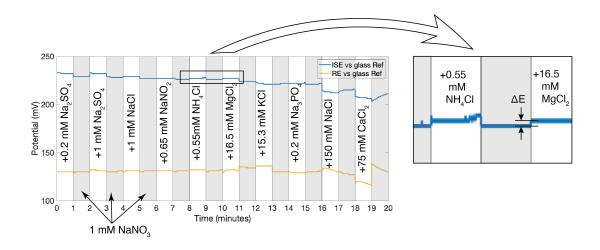
Figure 3.5: Potential over time of an ISE measured against a commercial reference electrode in solutions of various interfering ions (blue), and potential over time of a printed RE measured against a commercial reference (yellow). Both responses are stable with changing interference ions. (Inset)  $\Delta E$  is the potential difference between measurement in 1 mM NaNO<sub>3</sub> and measurement in solution containing an interfering ion.
