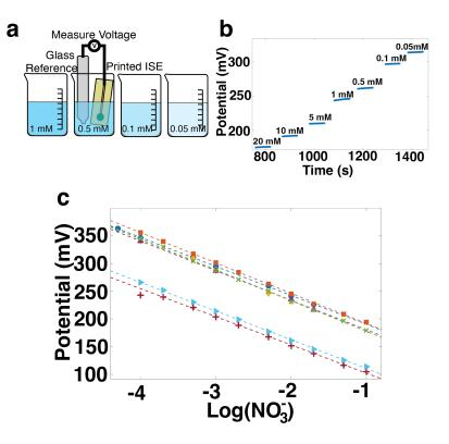
Figure 3.3: a) Characterization of a printed nitrate-selective electrode against a commercial reference electrode in NaNO<sub>3</sub> solutions of varying concentrations. b) Potential over time response of a printed nitrate-selective electrode in changing concentrations of nitrate. c) Sensitivity plot of 7 nitrate-selective electrodes overlaid, showing good repeatability and near-Nernstian response of  $-54.1 \pm 2.1 \text{ mV/dec}$ .
