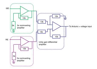
Figure 5.14: A three-part amplifier circuit for interfacing with potentiometric sensors. The ISE and RE are connected directly to op-amp terminals and see the input impedance of the op amp. Choosing op-amps with high impedance allows highimpedance measurement of sensors.
