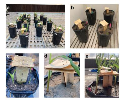
Figure 6.2: a) 16 pots with coated and uncoated bass and balsa wood stakes with corn growing in the greenhouse. b) 4 of the 8 wax-coated stakes with lettuce plants growing in the growth chamber. c) A wax-coated bass plywood sample is hydrophobic, so irrigation water beads up on the surface. d) An uncoated bass plywood sample absorbs water and the plies swell at different rates, leading to delamination. d) Complete delamination of the top ply of uncoated bass plywood.
