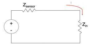
Figure 5.11: The nitrate sensor acts as a voltage source, driving a current through the measurement device.
