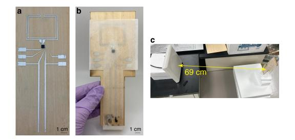
Figure 5.10: a) An AS3212 chip mounted on screen printed silver traces on a woodand-wax substrate. b) The same printed RFID tag with waxed paper encapsulation. c) Wirelessly reading data from the chip mounted on wood with waxed paper encapsulation.
