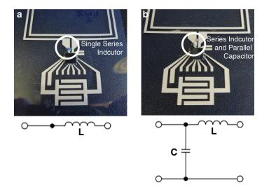
Figure 5.5: a) A single inductor in series between the chip and the antenna provides some matching. b) A series inductor and a parallel capacitor provide another degree of freedom and possible perfect impedance matching.
