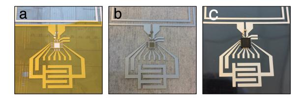
Figure 5.4: Rigid components are attached to to a screen-printed tag in three steps: (a) a laser cut stencil is used to define areas where (b) conductive ink is applied with a razor blade. (c) The components are placed with a pick-and-place tool.
