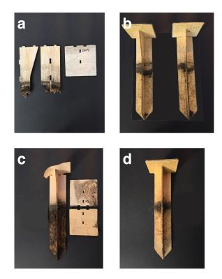
Figure 6.3: a)Balsa wood without wax encapsulation decomposed under the soil surface in 90 days. b) Balsa wood with beeswax encapsulation layer did not degrade. c) 3-ply bass wood delaminated above the soil level and began to decompose under the soil level. d) 3-ply bass wood with beeswax encapsulation did not degrade.
