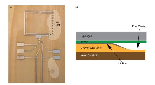
Figure 2.6: a) A substrate with uneven thickness has areas that did not print. b) A cross-sectional view of an uneven substrate illustrating how thickness variations can cause misprints like the one seen in (a).
