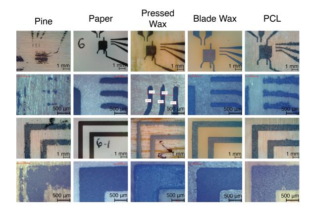
Figure 2.4: Although large features print decently well on all substrates, fine features and edge roughness are improved when printing on smoother substrates: blade coated wax, pressed wax, and PCL-coated wood as compared to raw wood or soaked wood.
