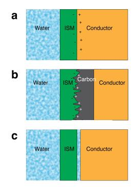
Figure 3.10: a) Simple coated-wire type ISE without a transducer layer between the ISM and the conductor. b) Adding a carbon transducer layer between the ISM and the conductor increases surface area, increases capacitance, and reduces water layer formation. c) A coated-wire type electrode can form a layer of water under the ISM, which causes drift.
