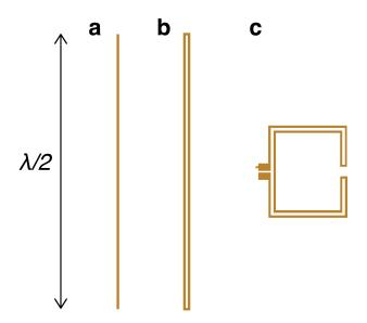
Figure 4.2: a) A standard half-wavelength dipole. b) A folded dipole is a very narrow loop of wire that is still a half-wavelength from end to end. Width and gap dimensions can be used to vary input impedance. c) The arms of the folded dipole can be bent in to form a more compact antenna.
