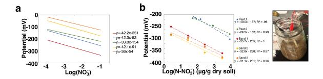
Figure 3.9: a) Sensitivity curves for five printed sensors using carbon ISEs. b) Potential versus nitrate concentration for two sensors in a high-organic-matter soil and three sensors in sand.
