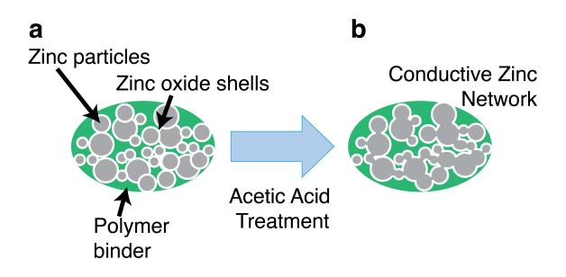
Figure 2.12: a) As-printed zinc ink consists of discrete zinc micro particles, each with an oxide shell. This matrix is not conductive. b) After treatment with a solution of acetic acid, which reacts with the oxide layer, a conductive network of zinc is formed. A new passivisation layer forms on the outside of network.
