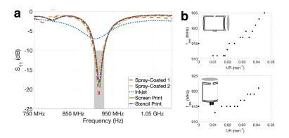
Figure 4.6: a) Power reflection coefficient (S11) parameters show that spray coated, stencil printed, and screen printed samples achieve good resonance (S11 ; -10 dB) in the targeted 902-928 MHz band, while inkjet printed samples have a much smaller resonance peak. b) Bending the antenna around a smaller radius shifts the resonance peak (frequency where S11 is the lowest) to higher frequencies. Up to radii of 20 mm, the peak stays within the 902-928 MHz band.
