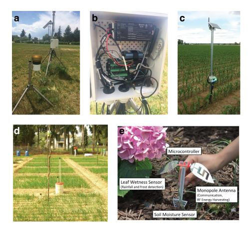
Figure 1.8: a) single-point weather station with a temperature, anemometer, solar radiation, rainfall, and other sensors wired to a central hub. b) The data logger and cellular up-link modem inside the hub of the weather station. c) A stand-alone soil moisture installation with solar power and cellular data upload capability. d) Cellular-based soil moisture sensors deployed at IIT Kharagpur from [31] e) inkjet printed soil moisture and leaf wetness sensor with RFID communication from [34].
