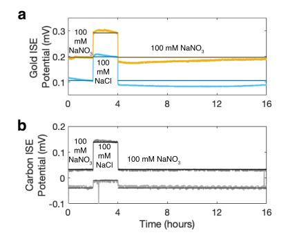
Figure 3.11: a) Water layer test with gold electrodes indicates formation of water layer. b) Water layer test with carbon electrodes shows more stable behavior.
