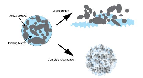
Figure 1.11: A composite material might experience disintegration if the binding matrix is made of a biodegradable material while the active material inside does not degrade. Complete biodegradation involves the molecular breakdown of all constituent parts.
