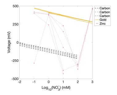
Figure 3.7: Carbon makes a good ISE. Zinc doesn't.
