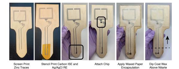
Figure 7.1: A prototype of a process for printing the full sensor node begins with substrate preparation, followed by zinc printing, nitrate sensor electrode printing, chip attachment, and two wax encapsulation steps.
