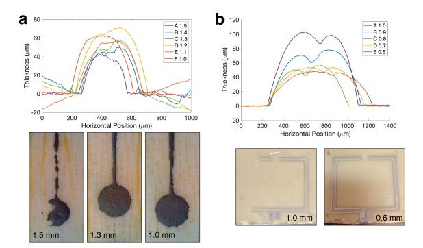
Figure 2.11: With well-adjusted snap off, the full pattern prints and thickness is uniform across the width of the printed trace. When snap off is too high, the thickness is greater, but the print is poorly controlled. a) 500  $\mu$ m wide traces of zinc on wax-soaked balsa wood with varying snap off. b) 1 mm wide traces of zinc on blade-coated wax substrates with varying snap-off.
