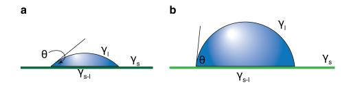
Figure 2.7: The amount of spreading of a drop of liquid, including inks, is determined by the surface tension of the liquid,  $\gamma_l$ , the surface energy of the solid-air interface,  $\gamma_s$ , and the energy at the surface between the solid and the liquid,  $\gamma_{s-l}$ . The contact angle of a drop on a solid surface is used to quantify surface energy. a) High surface energy, low contact angle substrate. b) Low surface energy, high contact angle substrate.
