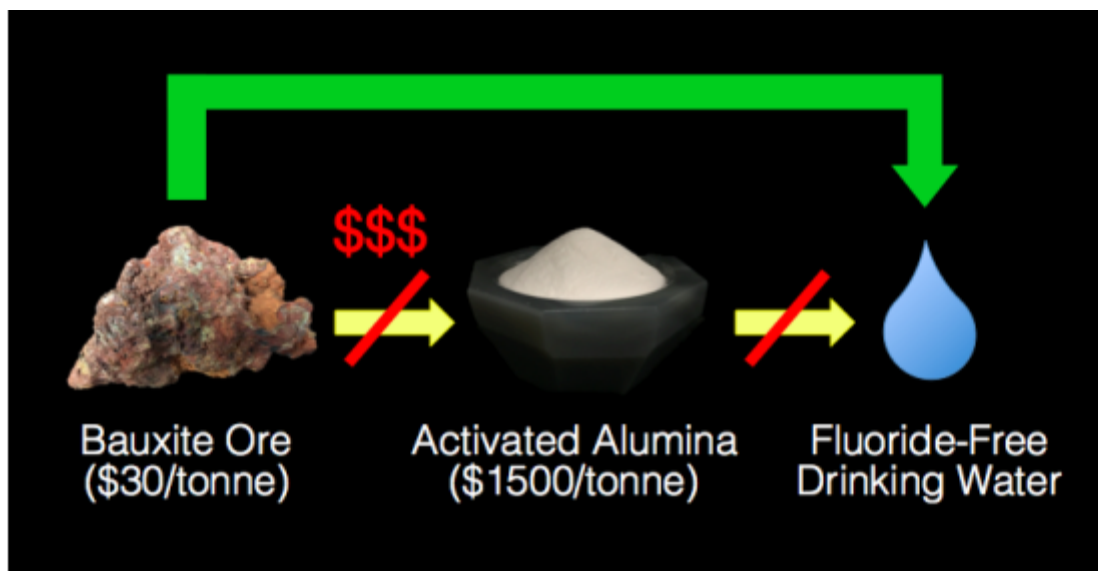
Figure 3. Flow diagram demonstrating cost savings associated with using raw bauxite as opposed to activated alumina as an adsorbent material for remediating fluoride contaminated groundwater.
