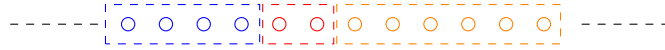
Figure 2.7: OSA illustration: points are ordered w.r.t. LLR values. Each color represents a cluster and LLR value difference in each cluster is less than l_s .
