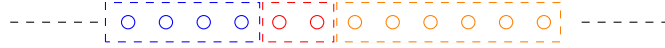
Figure 2.7: OSA illustration: points are ordered w.r.t. LLR values. Each color represents a cluster and LLR value difference in each cluster is less than l_s .
