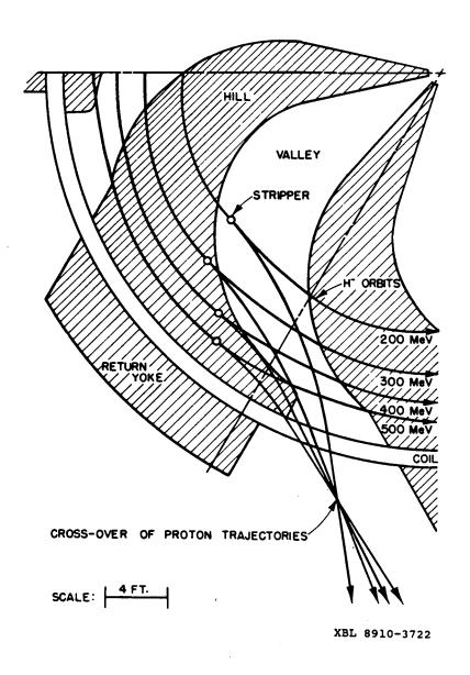
Fig. 5. The stripping used by TRIUMF for high efficiency extraction with  $H^-$  beams, giving high currents of 200  $\mu A$ .
