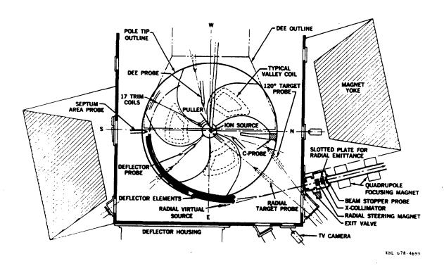
Fig. 2. LBL 88-Inch Cyclotron, a typical multiparticle, variable energy cyclotron with heavy ion beams up to 32 MeV/u. A Case 2 example.
