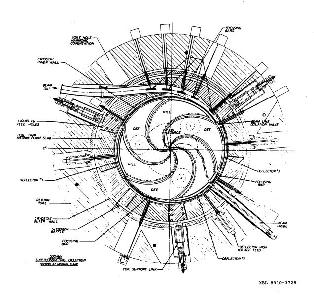
Fig. 6. Michigan State University K-500 superconducting cyclotron, Case 4. This is the most compact design, and lowest cost for high energies.
