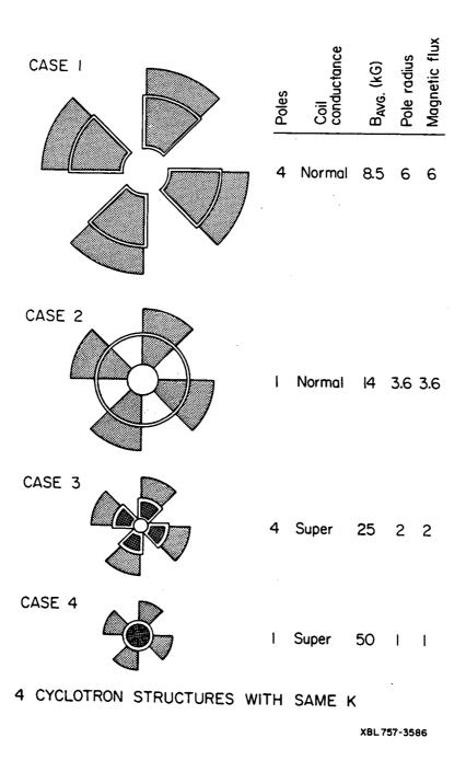
Fig. 1. Four cyclotron designs, showing relative scale. Single pole vs. separate sector and normal vs. superconducting.
