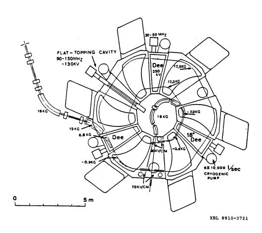
Fig. 3. The Osaka separate sector cyclotron, showing 6 magnet sectors, 3 dees and injection and extraction channels. A Case 1 example.
