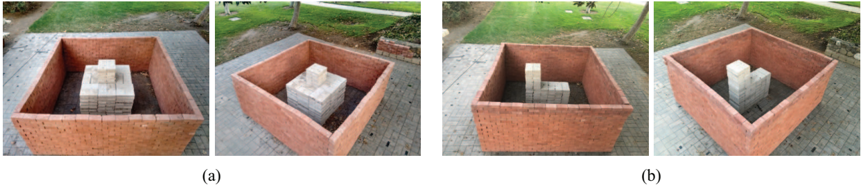
Figure 2.8: The two areas of interest for 3D through-wall imaging. (a) shows the two-cube scenario and (b) shows the L-shape scenario. For better clarity, two views are shown for each area.
