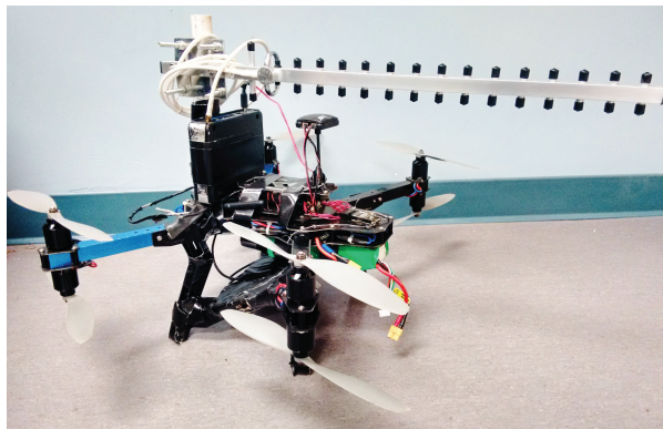
Figure 2.7: A 3DR X8 octo-copter used in our experiments.
