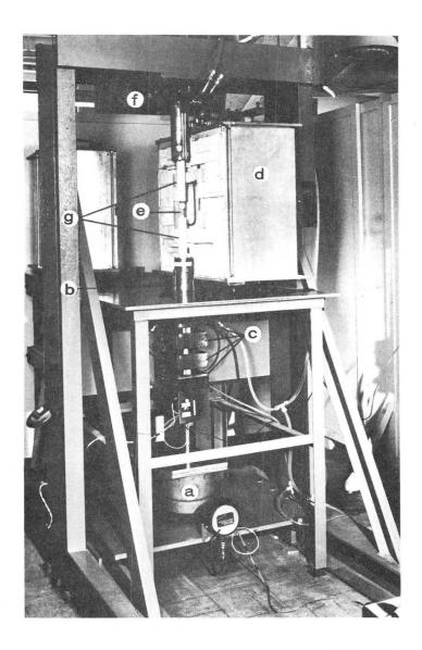
Fig. 3. Compressive deformation Apparatus III: a: diaphragm cylinder; b: loading column; c: alignment bushings; d: half of furnace; e: specimen; f: triangular alignment plate; and g: Al<sub>2</sub>O<sub>3</sub> rams.
