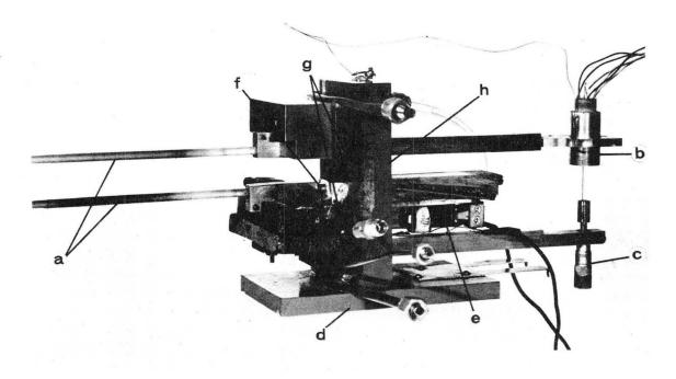
Fig. 9. Strain-measuring device for Apparatus II: a: sapphire rods; b: linear differential transformer; c: Invar micrometer supporting transformer core; d: spring-loaded platform; e: buzzer; f: spring-loaded shaft in lower lever; g: pivot bearings; and h: Invar pivot support frame.
