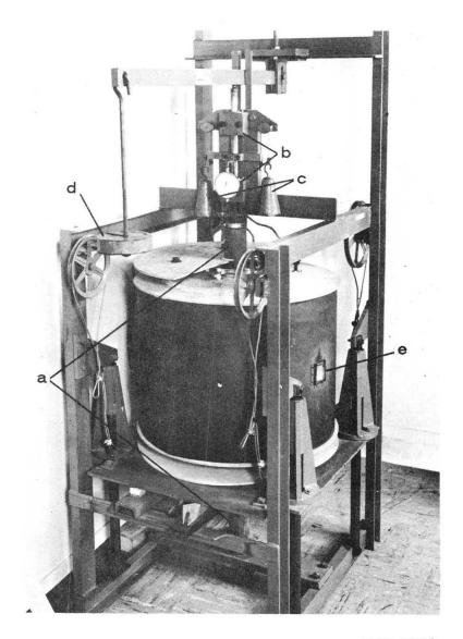
Fig. 1. Compressive deformation Apparatus I: a: SiC loading rams; b: alignment bushings for upper movable ram; c: counterweights for upper ram; d: loading weight; and e: Vycor window in Globar furnace for measurement of deformation.
