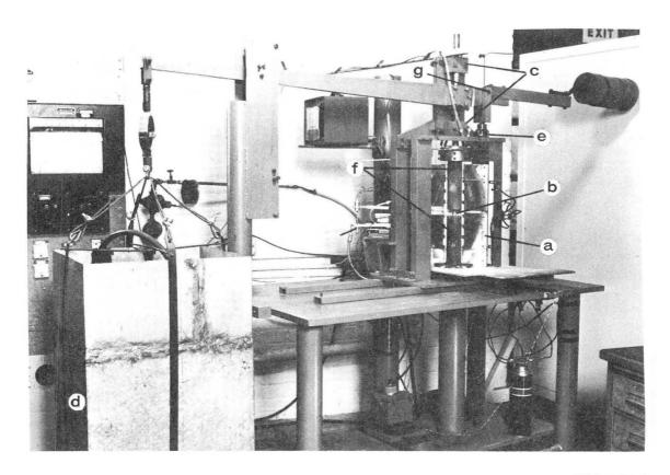
Fig. 2. Compressive deformation Apparatus II: a: half of furnace; b: specimen; c: alignment bushings; d: loading tank; e: universal joint; f: SiC rams; and g: lever fulcrum.
