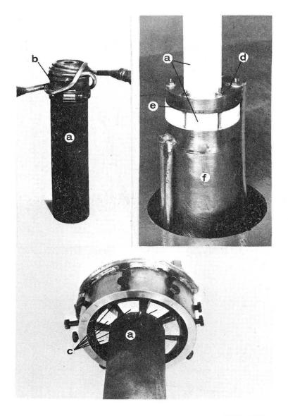
Fig. 5. Compression ram attachments to the metal alignment system: a: compression rams; b: water-cooled slotted steel cup; c: Transite pieces; d: internally water-cooled ring; e: copper gasket; and f: main steel loading column.
