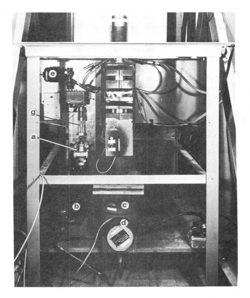
Fig. 7. Photograph of hydraulic loading system for Apparatus III.
