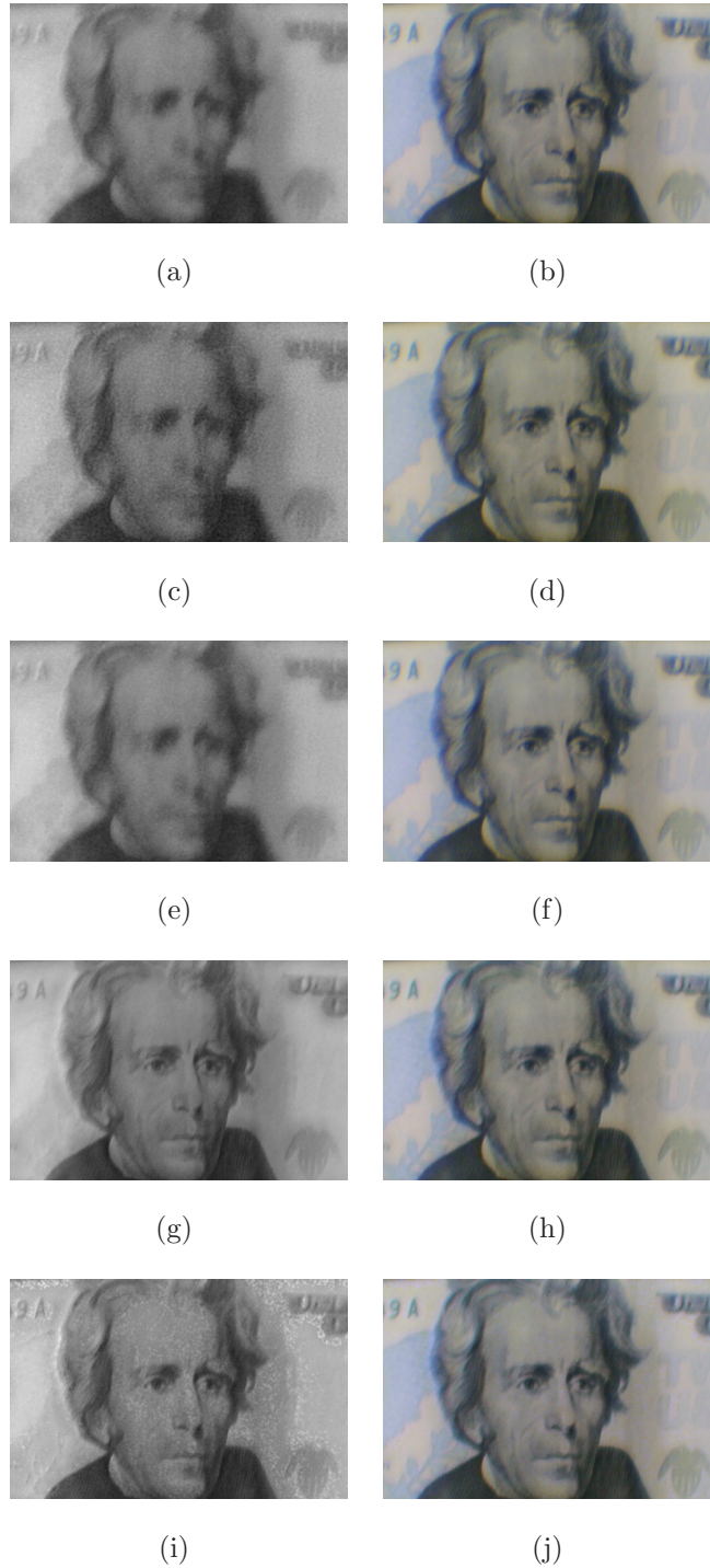
Figure 6.17: These image were taken using the FLCS in a lab setting. The color images must be viewed in color. (a) Original blue image; (b) original color image; (c) Wiener blue image; (d) Wiener color image; (e) Lucy-Richardson blue image; (f) Lucy-Richardson color image; (g) contourlet blue image; (h) contourlet color image; (i) proposed blue image; (j) proposed color image.
