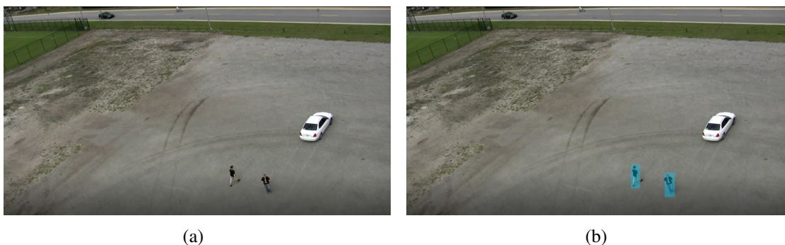
Figure 2.11. A UAV image a) before and b) after applying the DNN based object detection.
