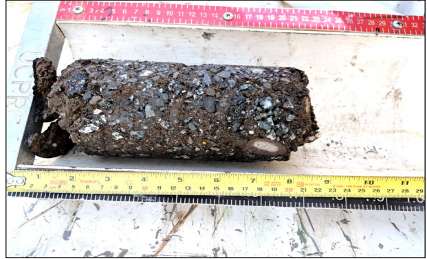
Figure 6.21: Core taken from area with no surface distress.
