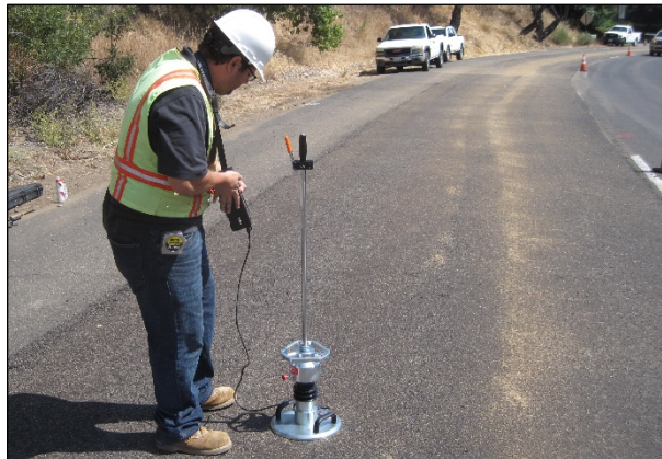
Figure 3.12: Light weight deflectometer.
