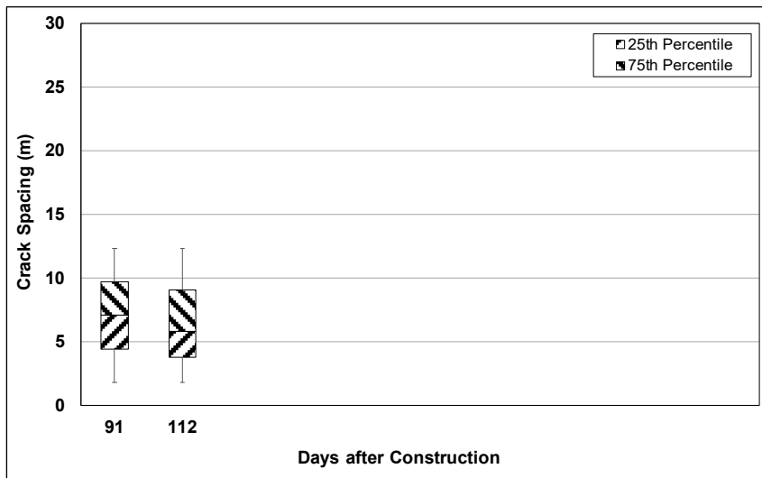
Figure B.39: Cell S5: Change in crack spacing.
