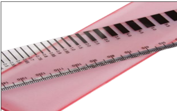
Figure 2.24: Crack width gauge.
