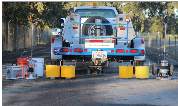
Figure 5.21: Stiffness measuring equipment used on the FDR-C Test Road. (FWD, SSG, and LWD).
