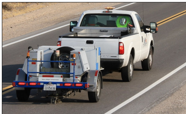
Figure 3.11: Falling weight deflectometer.
