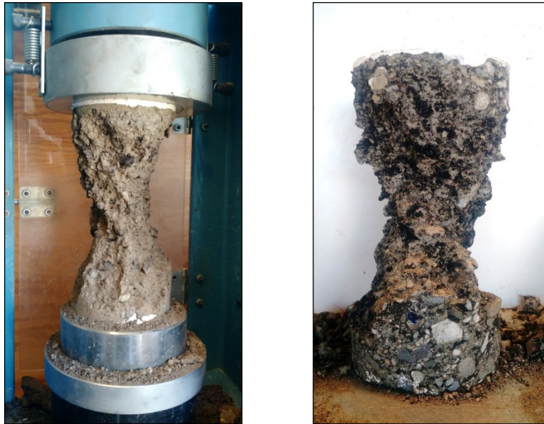
Figure 3.16: Typical hour glass shear failure of FDR specimens after UCS testing.
