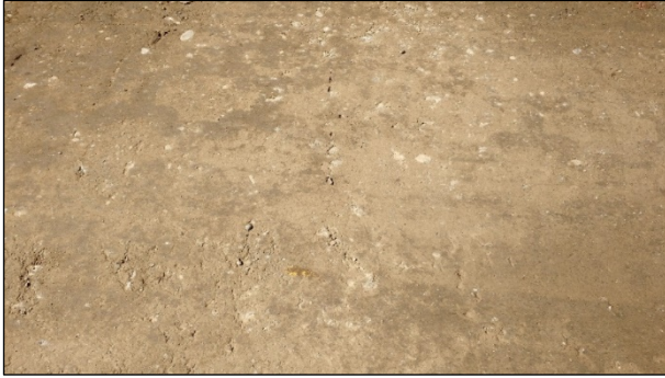
Figure 5.31: Surface condition after three passes with SSR at high vibration amplitude.
