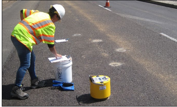
Figure 3.13: Soil stiffness gauge.
