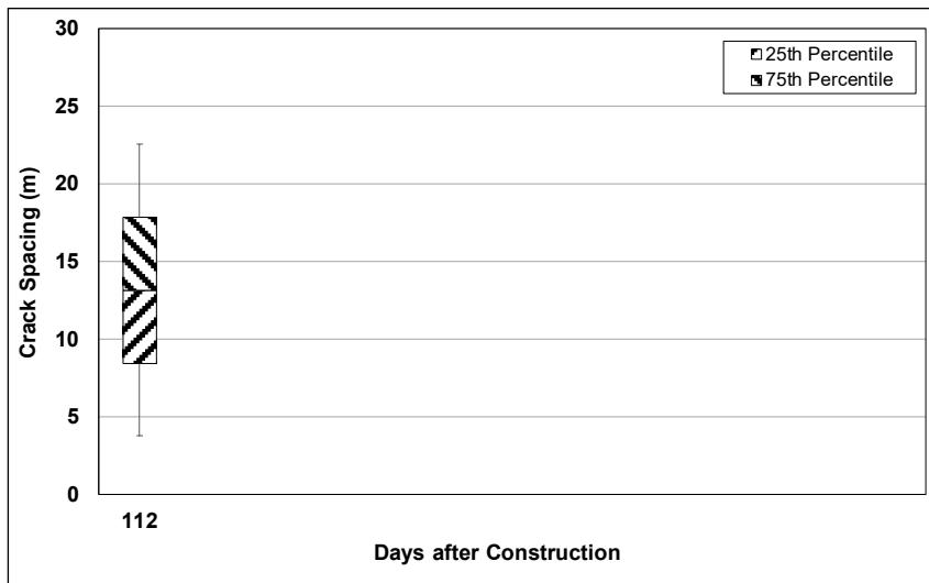
Figure B.30: Cell S4: Change in crack spacing.
