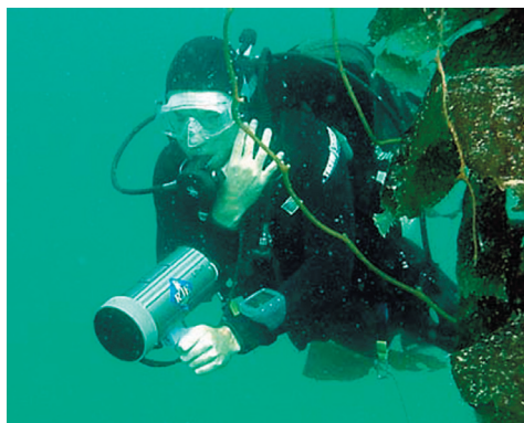
Left: Sea Grant trainee Darin Topping using an underwater receiver to follow sheephead fed an acoustic transmitter. This technique allows for assessment of behavior without the trauma associated with catching. Below: Topping displaying mature sheephead. Photos: Christopher Lowe
