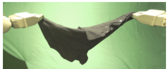
Fig. 10: A cloth configuration in which the article is flipped over itself and therefore not in the minimum-energy configuration that is predicted by our simulator.
