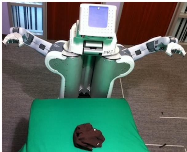
Fig. 1: The PR2 with a pair of pants in a crumpled initial configuration.
