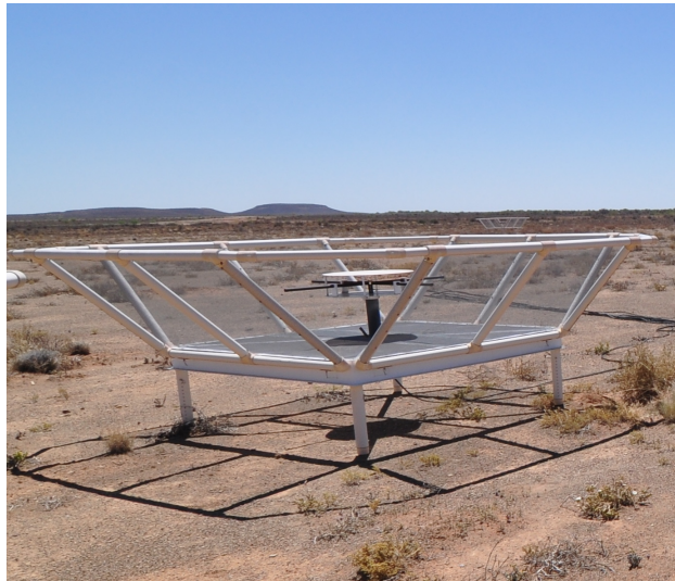
Figure 1.6: A PAPER antenna in the Karoo Desert in South Africa. A dual-polarization dipole sits at the center, surrounded by wire mesh panels that measure 2 m on each side.
