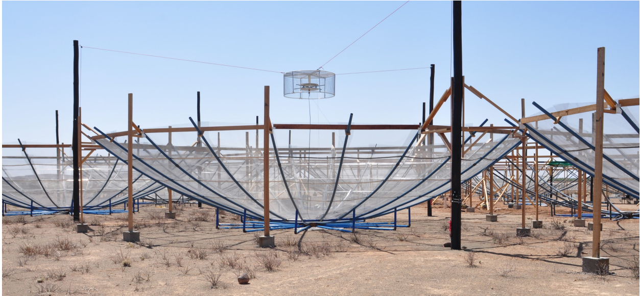
Figure 1.7: A HERA dish in the Karoo Desert in South Africa. Wire-mesh, PVC pipes, and wooden structures serve as the foundation for the 14 m diameter parabola. A PAPER dipole is suspended upside-down with a wire pulley-system and surrounded by a prototype wire-mesh skirt structure. HERA-350 will use an updated design for its feed; however, HERA’s initial data releases use the old PAPER infrastructure as depicted here.
