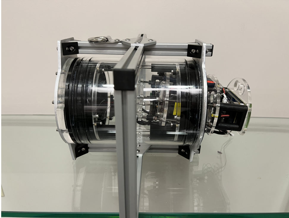
Figure 4.5: FishSense Version 2 prototype with the electronics rack half-removed.
