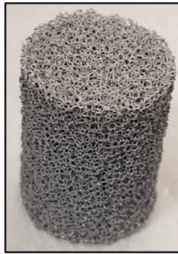
Figure 3.2: Image of prepared 3/4" x 1" cylindrical SiC reticulated foam sample. SiC foams were provided and manufactured by Ultramet using chemical vapor deposition onto preforms.
