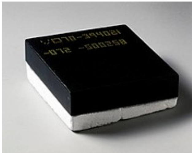
Figure 1.2: Image of thermal insulation tiles used for the Space Shuttle.
