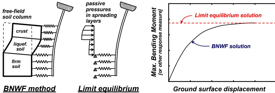
Fig. 2. Schematic comparison of limit equilibrium and BNWF methods.
