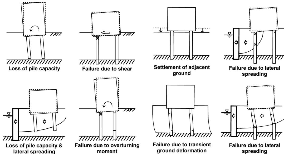
Fig. 1. Schematics of pile damage mechanisms in liquefied ground (modified from Tokimatsu et al. 1996).
