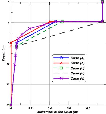
Fig. 11. Different assumed soil displacement profiles for parametric study of pushover analysis method.
