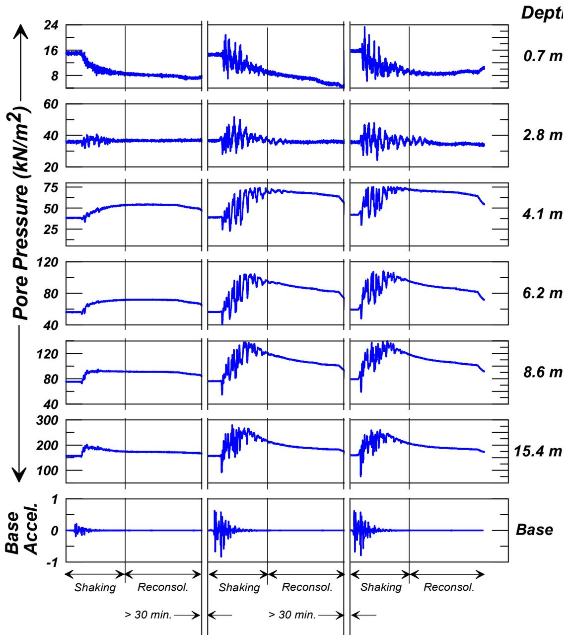
Fig. 7: Pore pressure time histories for a vertical array of pore water pressure transducers near the center of the model container for PDS01.
