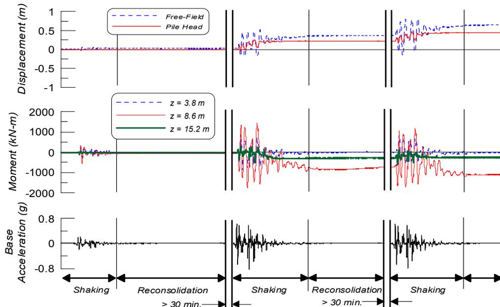
Fig. 8. Displacement, moment and base acceleration time histories for the medium-sized single pile. Z is measured from the ground surface.
