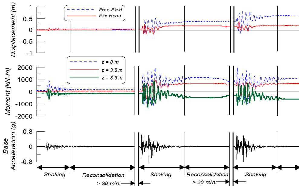
Fig. 9. Displacement, moment and base acceleration time histories for the upslope pile in the 2-pile group. Z is measured from the ground surface.
