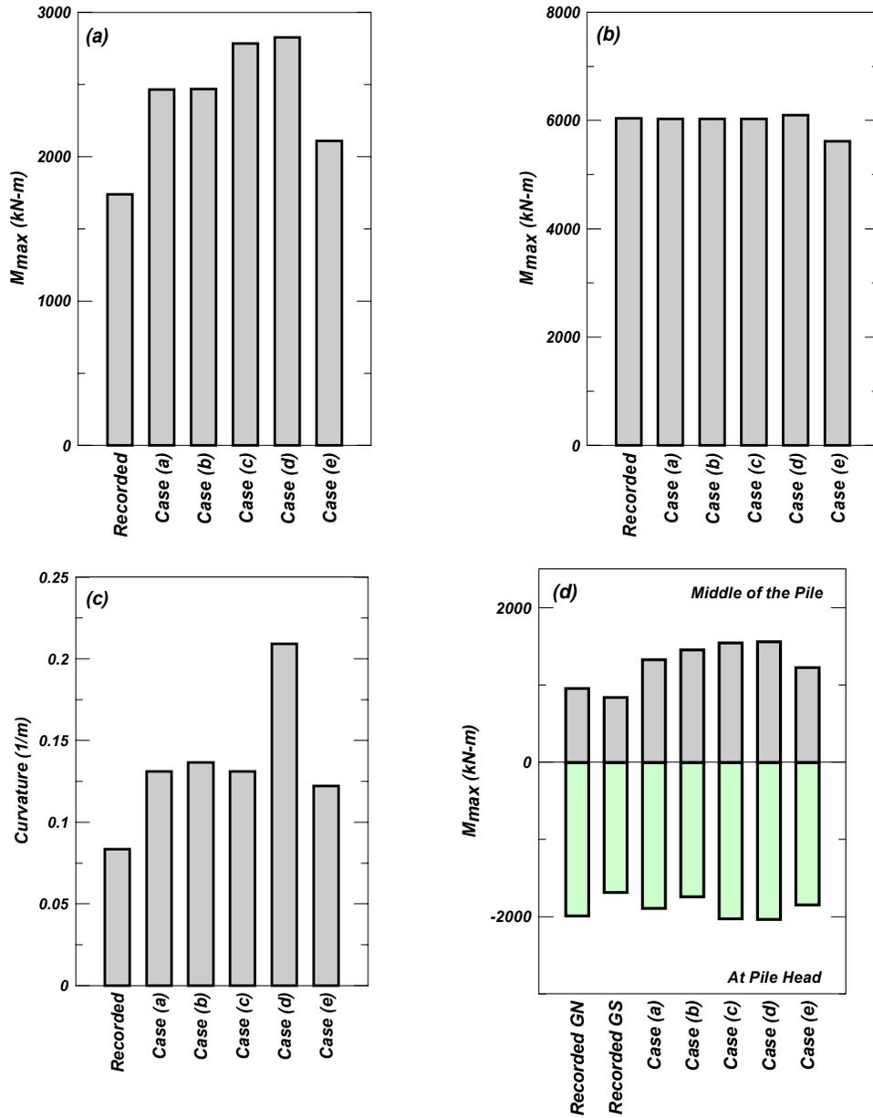
Fig. 14. Comparison of calculated and recorded maximum moments: (a) MP, (b) BP, (c) SP, (d) GP
