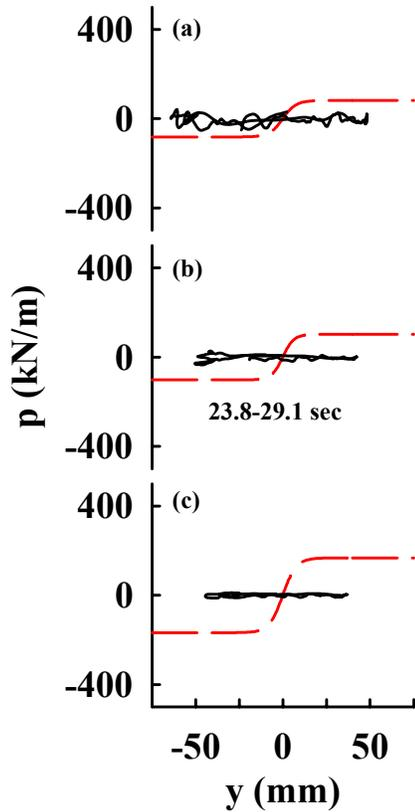
Fig. 3. p-y loops in liquefying loose sand ( $D_r \approx 40\%$ ) at depths (a) 2-D, (b) 3-D, and (c) 4-D ( $D = 0.67$  m). Dashed lines per API (1993). (Wilson et al. 2000)
