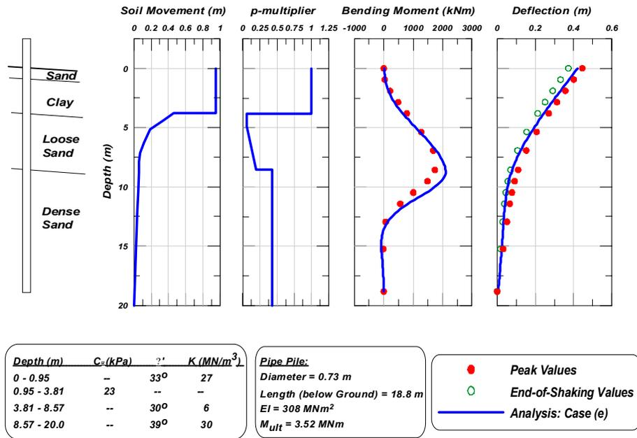
Fig. 13. Calculated and measured responses of the single middle-sized pile for case (e).
