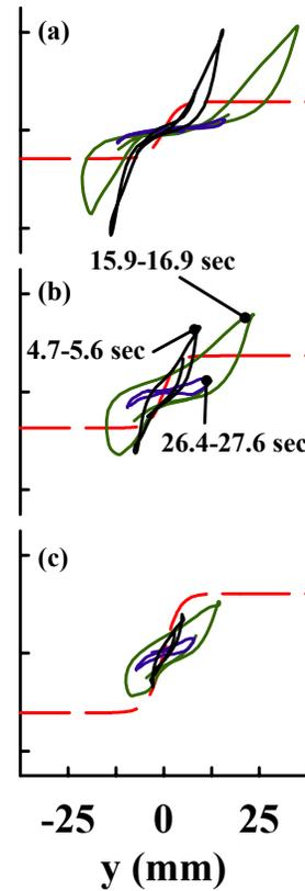
Fig. 4. p-y loops for liquefying med. sand ( $D_r \approx 55\%$ ) at depths (a) 2-D, (b) 3-D, and (c) 4-D ( $D = 0.67$  m). Dashed lines per API (1993). (Wilson et al. 2000)
