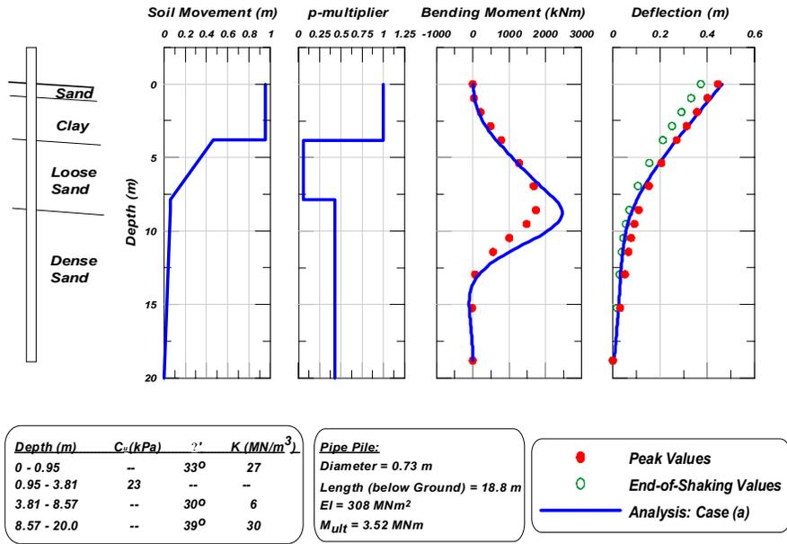
Fig. 12. Calculated and measured responses of the single middle-sized pile for case (a).
