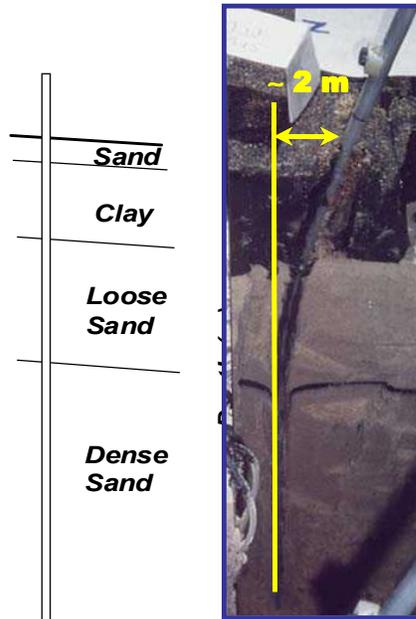
Fig. 10. Photo of deformed 0.36-m-diameter SP pile exposed during excavation of model after testing, with accompanying schematic of soil profile.
