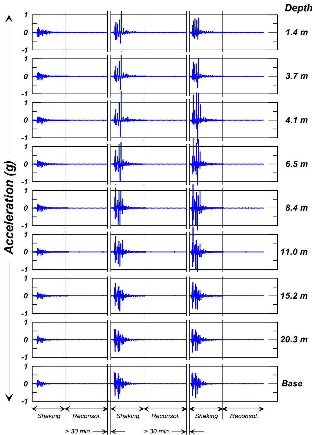
Fig. 6: Acceleration time histories for a vertical array of accelerometers located near the center of the model container for PDS01.
