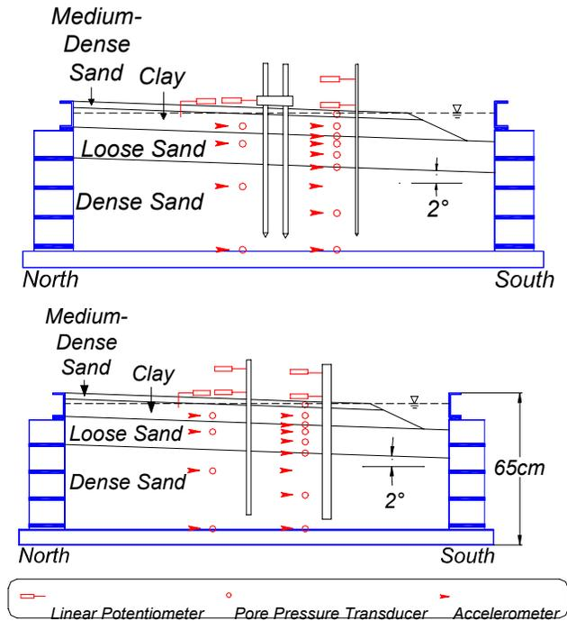
Fig. 5. Cross-sections of centrifuge model (west on top, east on bottom).
