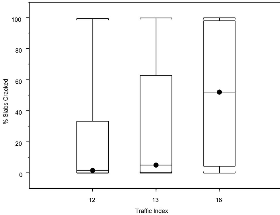
**Figure 8. Effect of traffic volume on transverse cracking.**
