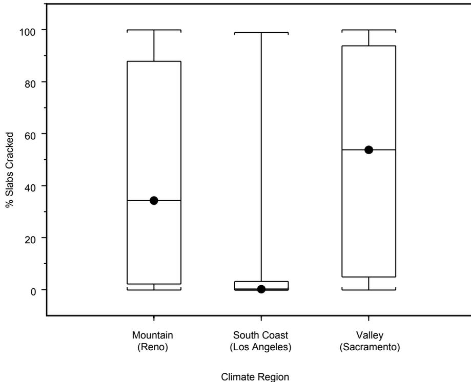
**Figure 7. Effect of climate region on transverse cracking.**
