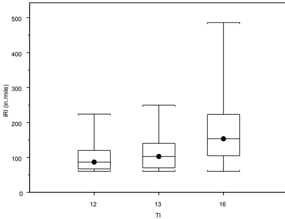
**Figure 28. Effect of traffic index (TI) on IRI.**
