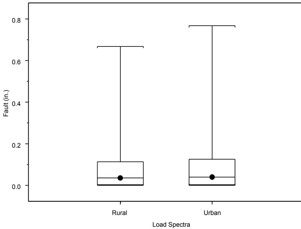
**Figure 23. Effect of load spectra on faulting.**
