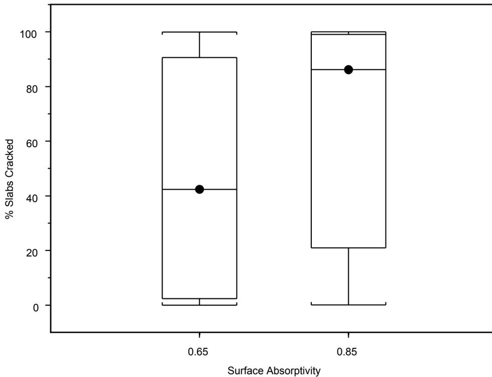
**Figure 41. Effect of surface absorptivity on transverse cracking.**
