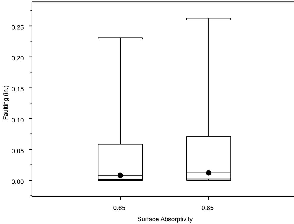
**Figure 42. Effect of surface absorptivity on faulting.**
