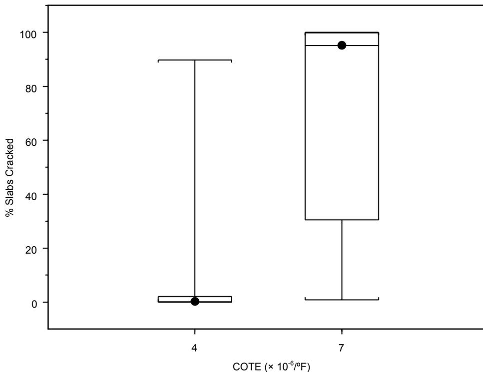
**Figure 38. Effect of COTE on transverse cracking.**
