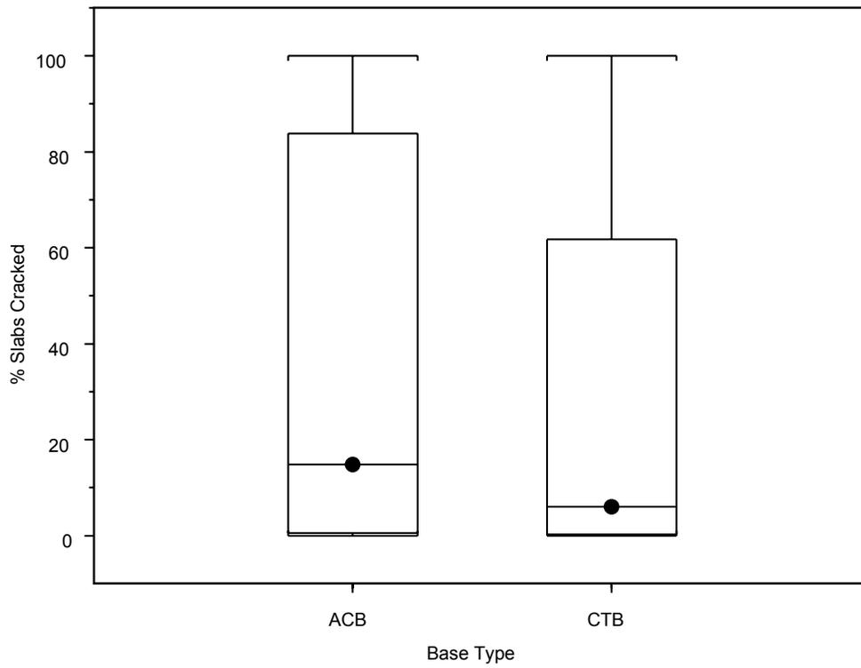
**Figure 11. Effect of base type on transverse cracking.**
