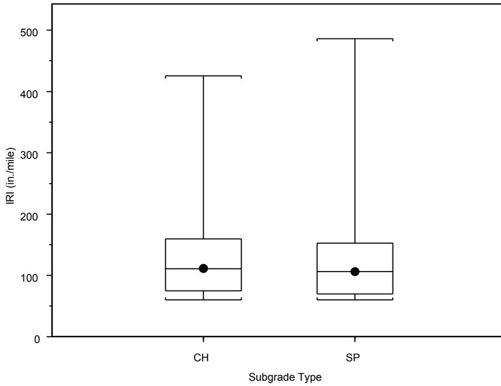
**Figure 33. Effect of subgrade type on IRI.**
