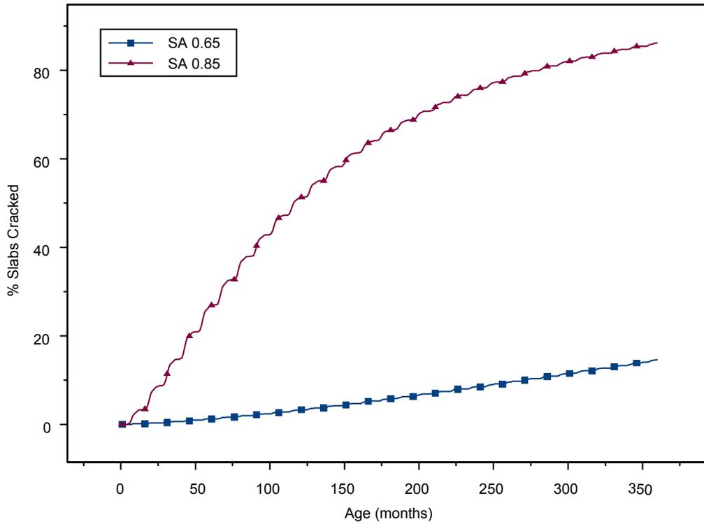
**Figure 40. Effect of the effect of surface absorptivity on transverse cracking (urban load spectra, 15-ft. joint spacing, wide truck lane, cement treated base, 8-in. PCC slab, design life of 30 years, and a reliability level of 50%).**
