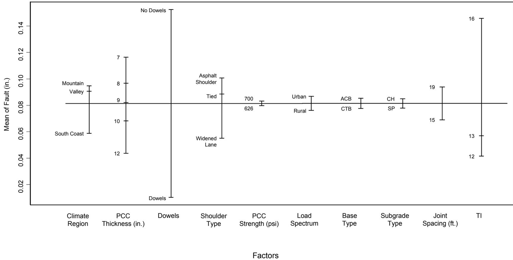
Figure 25. Relative effect of all variables on faulting.
