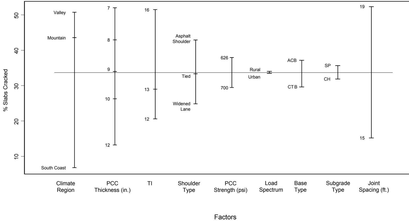
Figure 14. Relative effect of all variables on transverse cracking.
