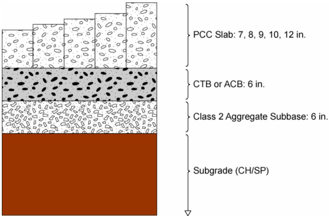
Figure 3. Pavement structure used for the sensitivity study.
