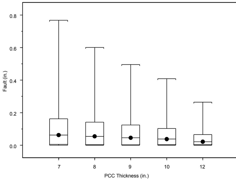
**Figure 17. Effect of PCC thickness on faulting**
