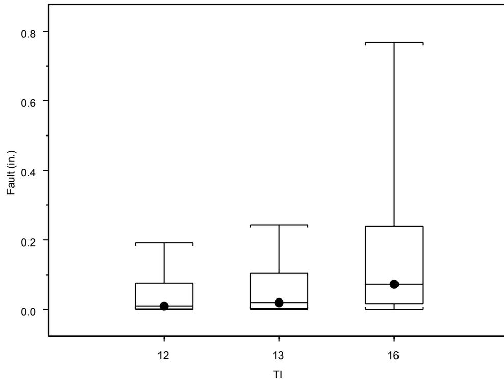
**Figure 18. Effect of traffic index (TI) on faulting.**
