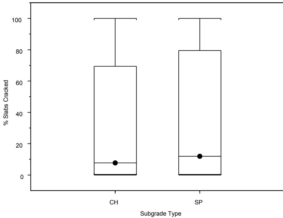
**Figure 9. Effect of subgrade type on transverse cracking.**
