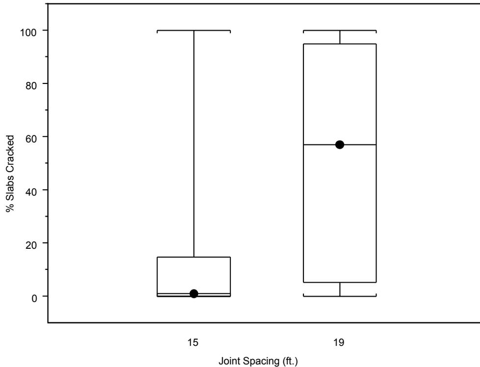
**Figure 6. Effect of joint spacing on transverse cracking.**
