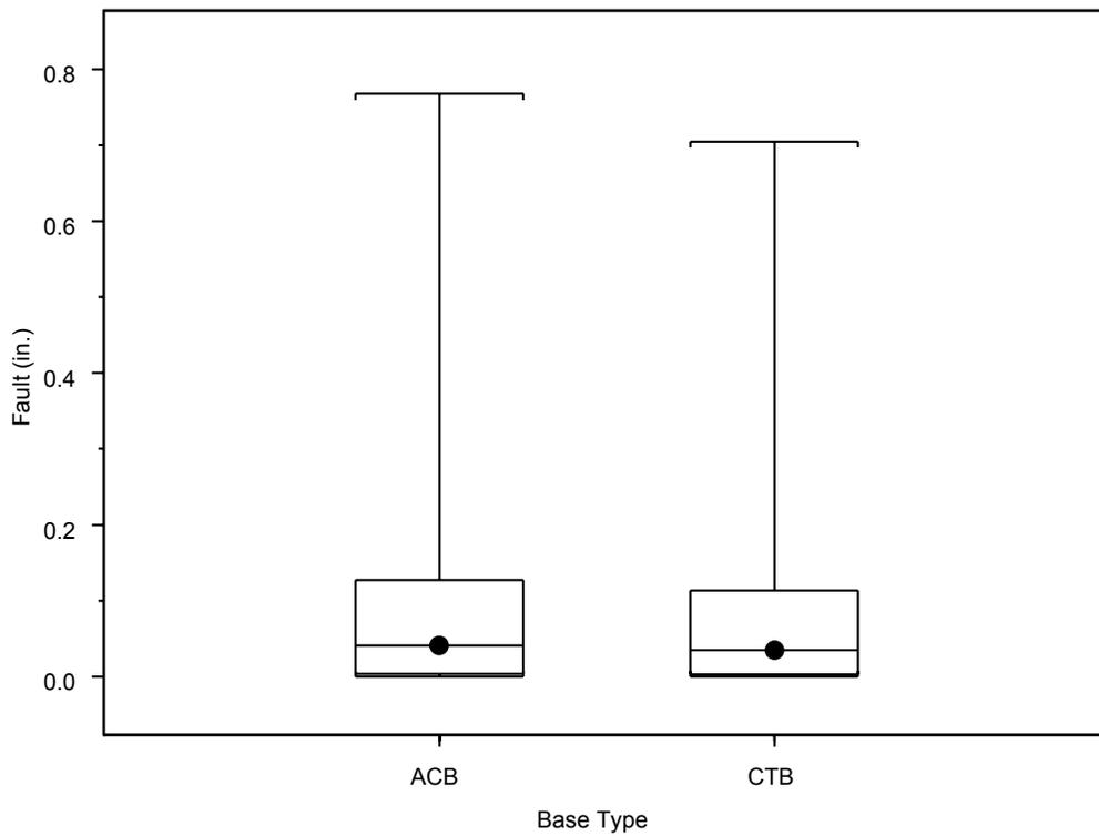
**Figure 21. Effect of base type on faulting.**
