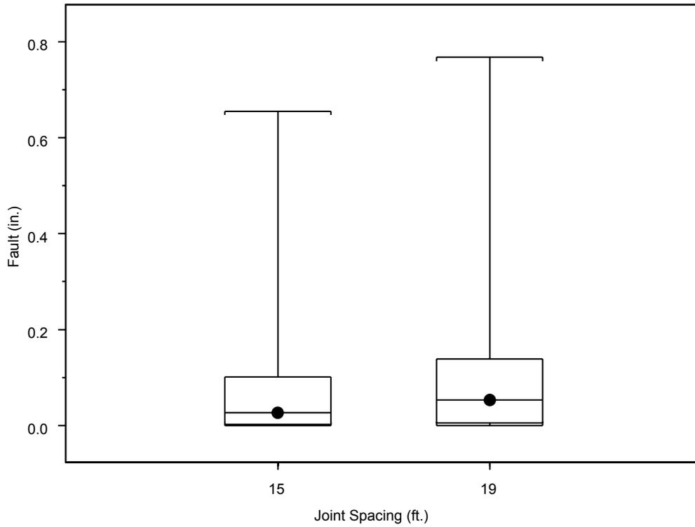
**Figure 20. Effect of joint spacing on faulting.**
