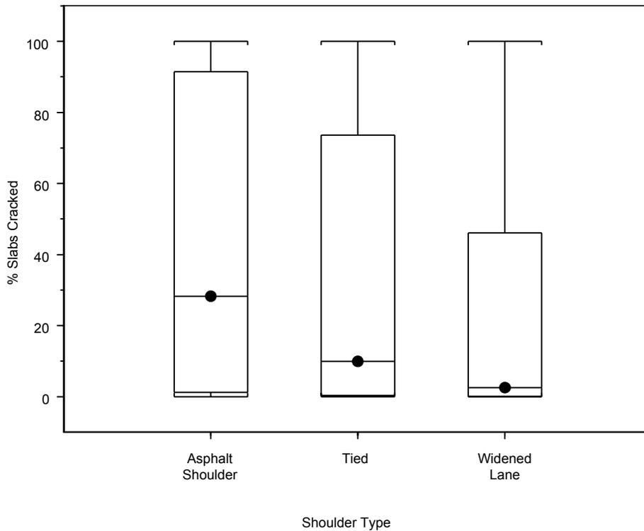
**Figure 5. Effect of shoulder type on transverse cracking.**
