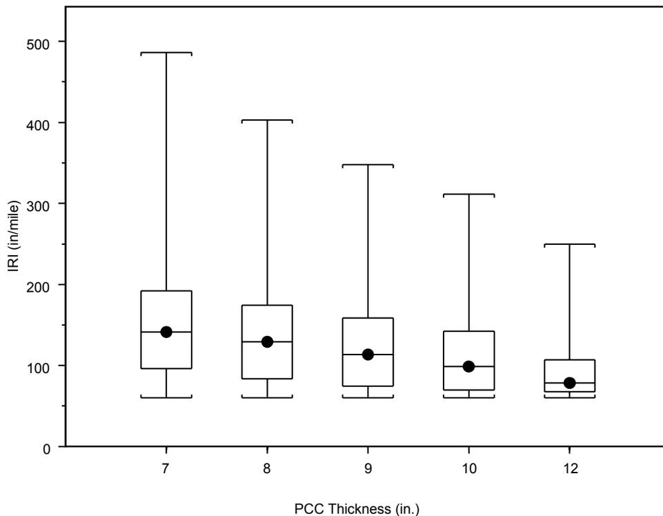
**Figure 26. Effect of PCC thickness on IRI.**
