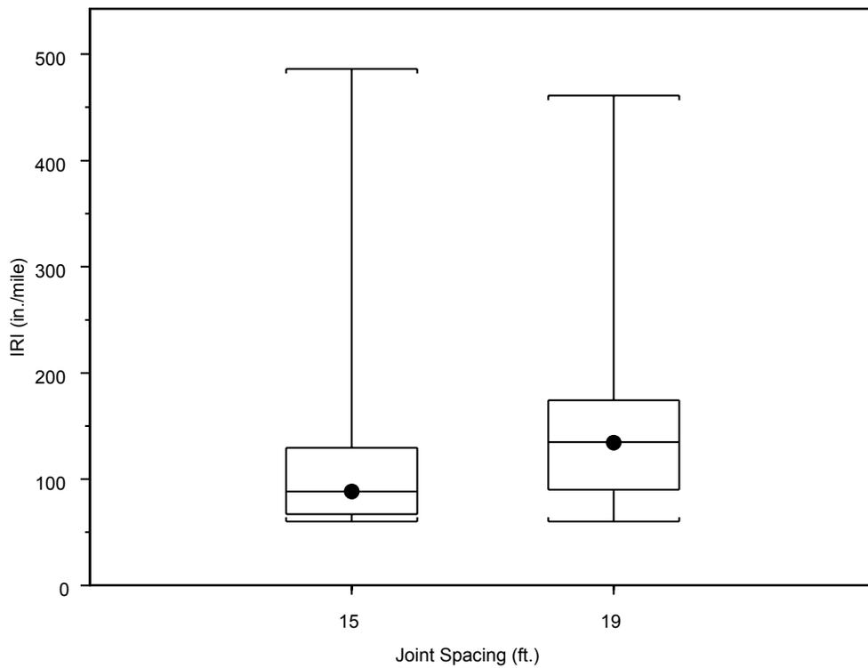
**Figure 30. Effect of joint spacing on IRI.**
