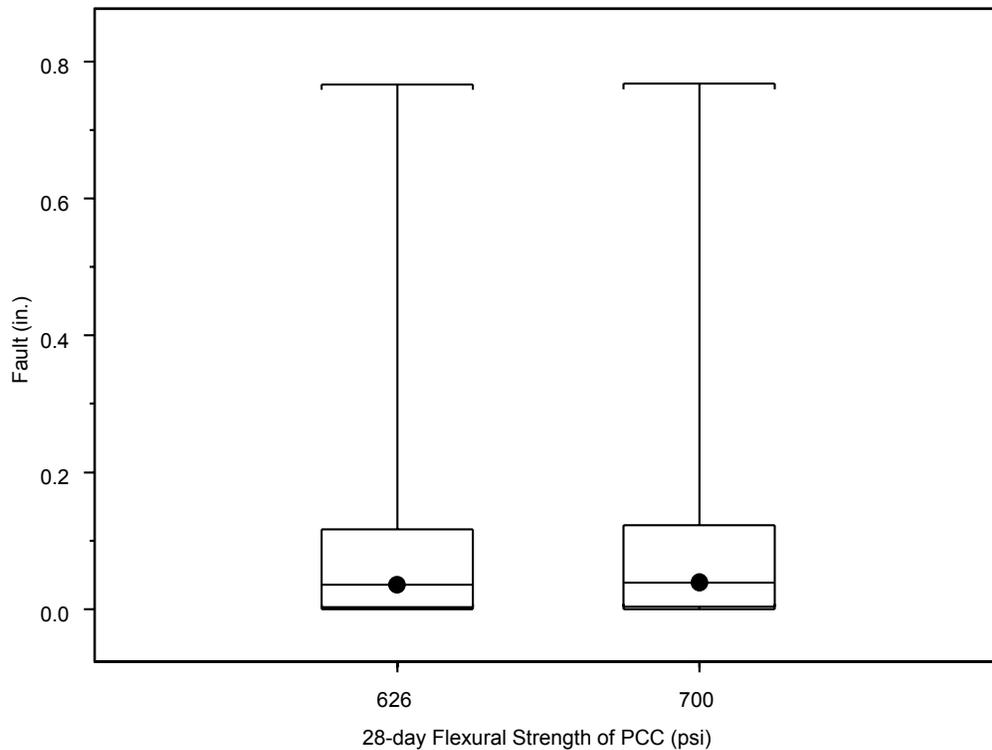
**Figure 24. Effect of PCC flexural strength on faulting.**
