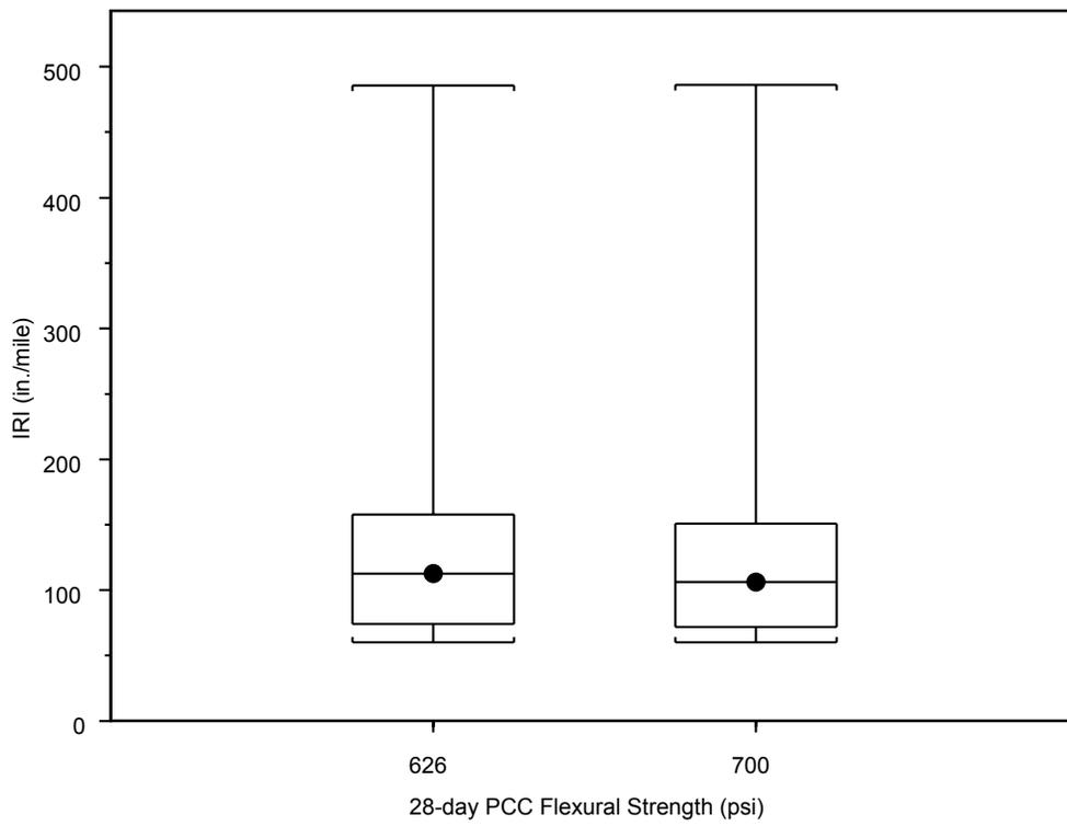
**Figure 34. Effect of PCC flexural strength on IRI.**
