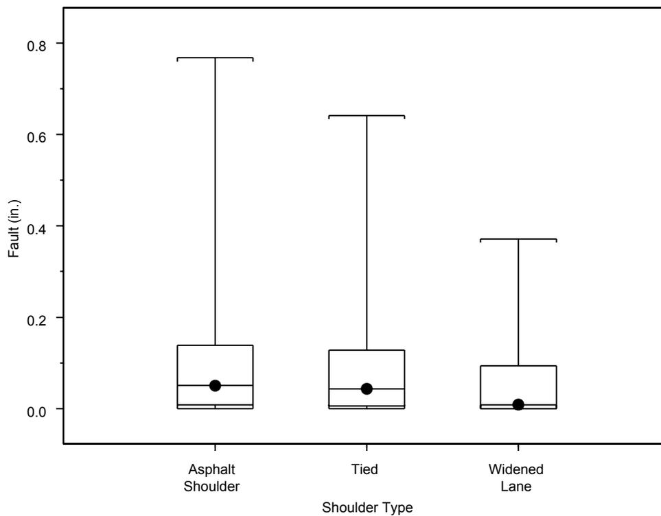
**Figure 19. Effect of shoulder type on faulting.**
