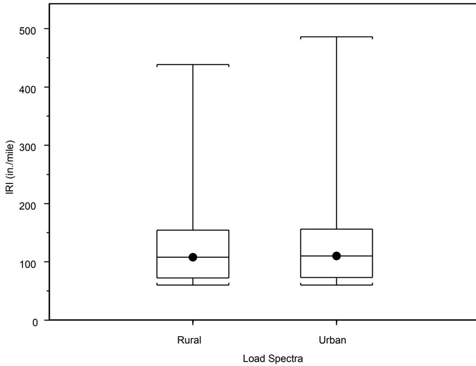
**Figure 31. Effect of load spectra on IRI.**
