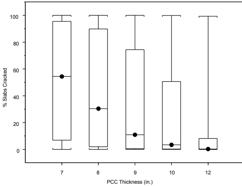
**Figure 10. Effect of PCC thickness on transverse cracking.**
