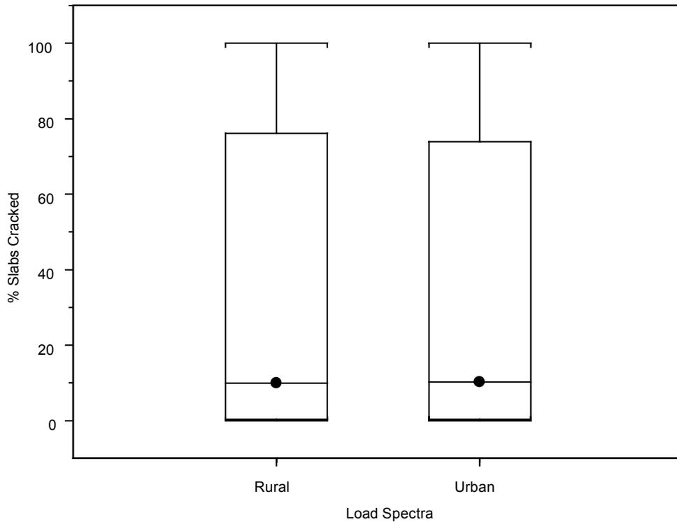
**Figure 12. Effect of load spectra on transverse cracking.**
