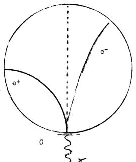
resolution around the circumference can be calculated or corrected by varying the geometry of the detectors. A 1.5 Bev electron is deflected 26° in a field of 20 kilogauss, in the 40-inch magnet.
