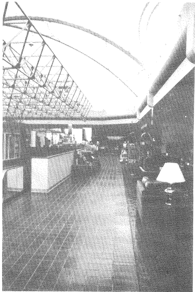
Softly diffused daylight through a tensioned fabric roof bathes the merchandising area of a Bullock's department store in San Jose, California. High daylight levels eliminate the need for electric light and are advantageous to merchandise display.
