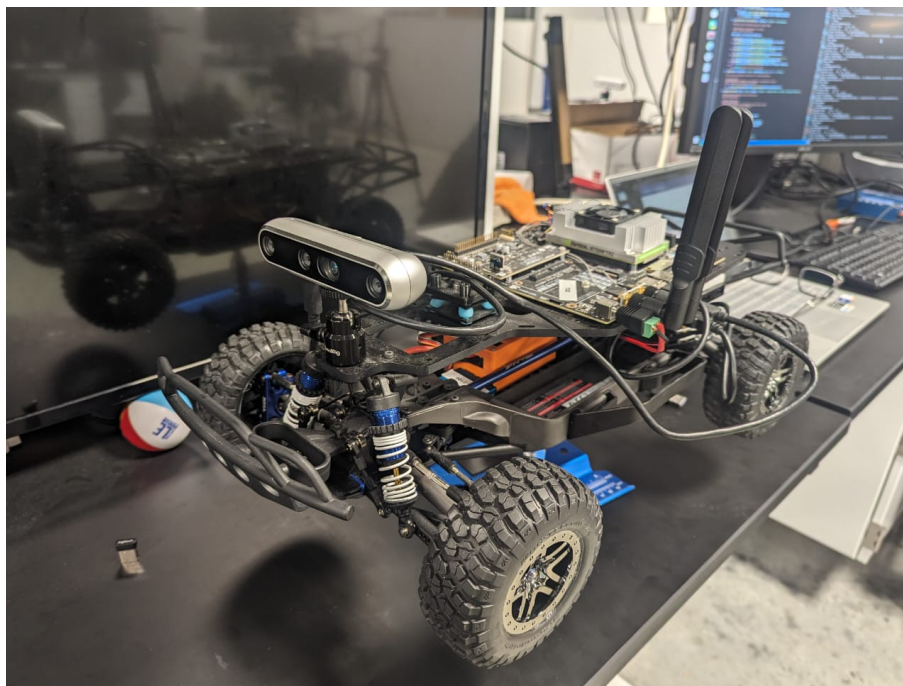
Figure 5.17. F1-tenth car used in real world experiments
