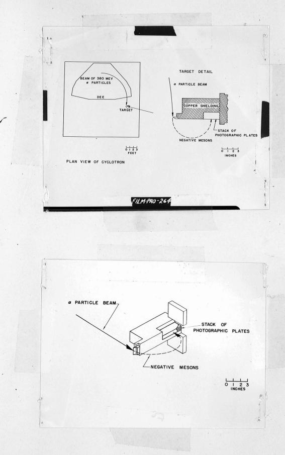
The next slide shows a photograph of the apparatus used for detecting negative mesons (photographic plates not shown)
