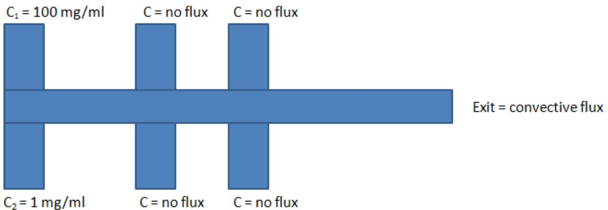
Figure 43: Convection-diffusion boundary conditions
