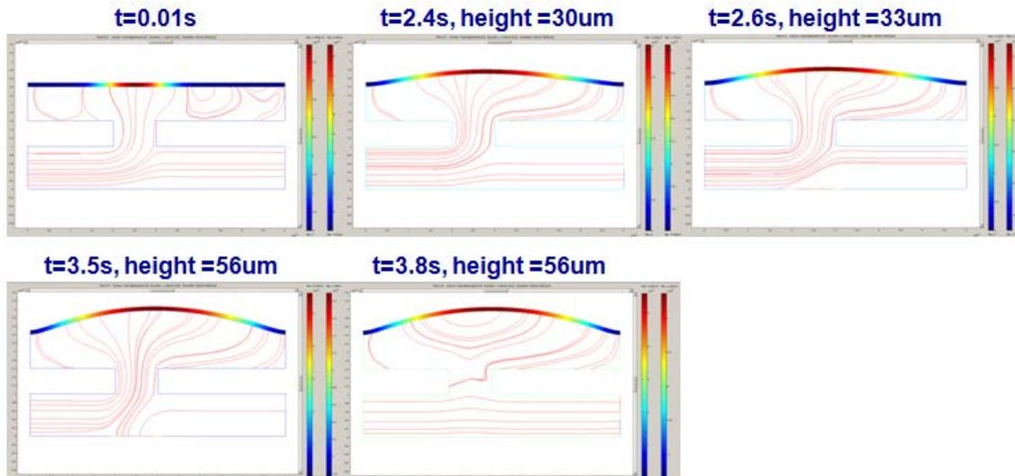
Figure 36: deformation of a PDMS membrane versus time.
