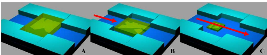
Figure 26. Conceptual schematic of heat activated microvalve. Hydrogel structures are patterned in situ using lithography (A). Heating the gel induces the gel to shrink (B) and open the valve (C).
