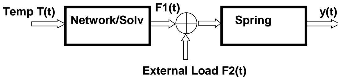
Figure 16: Active and passive components of gel model
