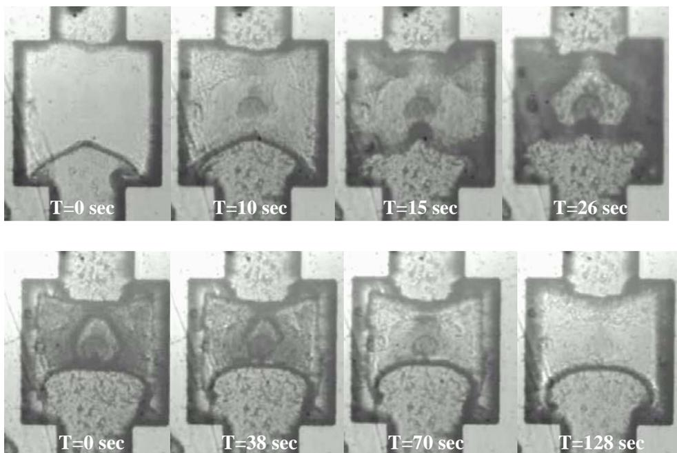
Figure 27. Collapse and expansion of a 200  $\mu\text{m}$  x 200  $\mu\text{m}$  x 75  $\mu\text{m}$  hydrogel valve. Series A shows the opening of a valve as heat is applied. Series B depicts the closing of the valve as the gel swells via diffusion
