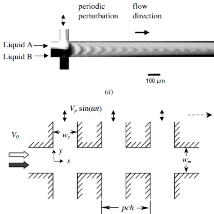
Figure 39: perturbation driven micromixers from Ref 33
