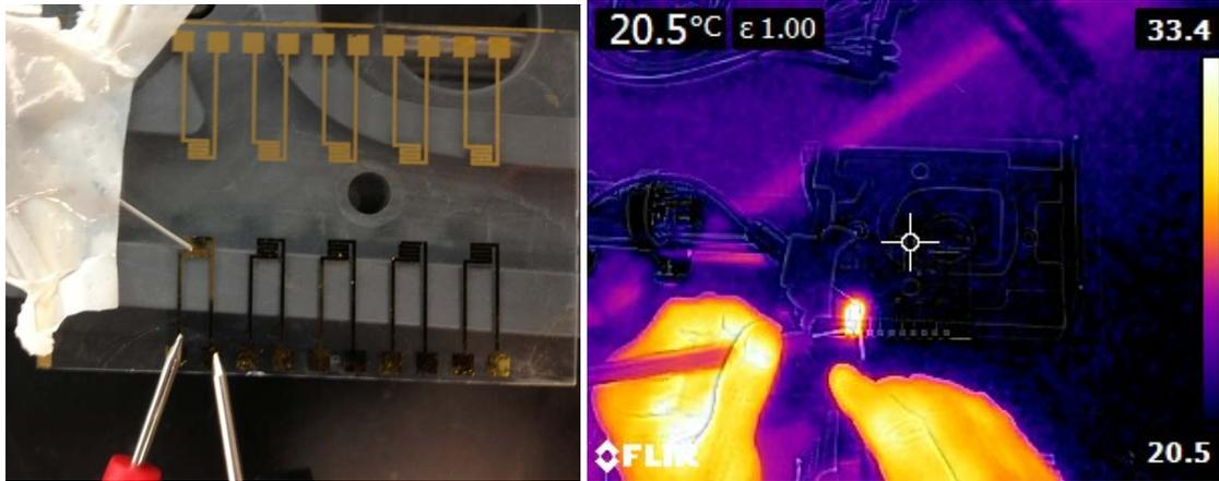
Figure 33: fabricated heaters and thermal imaging of heater
