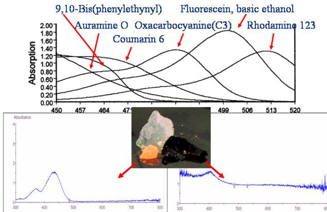
Figure 13: Novel light-sensitive gels and their absorbance spectra
