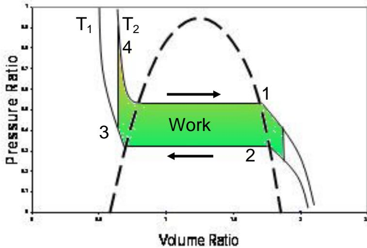
Figure 18: P-V diagram for a gel-based engine
