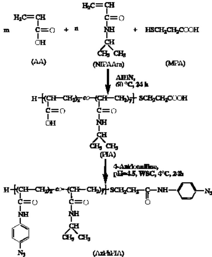
Figure 20: Synthesis of a lithographic NIPA hydrogel from Chen, Imanishi, and Ito
