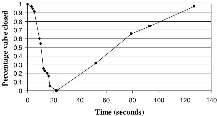
Figure 28. Gel valve opening and closing via water release and absorption versus time
