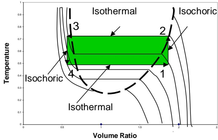
Figure 17: T-V diagram for a gel-based engine
