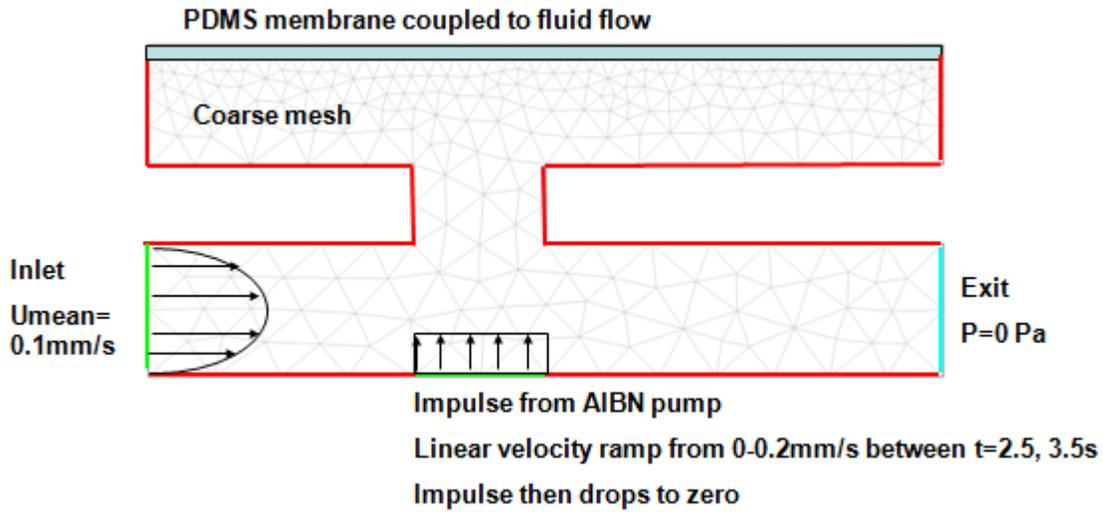
Figure 35. Analysis conditions and applied finite-element mesh
