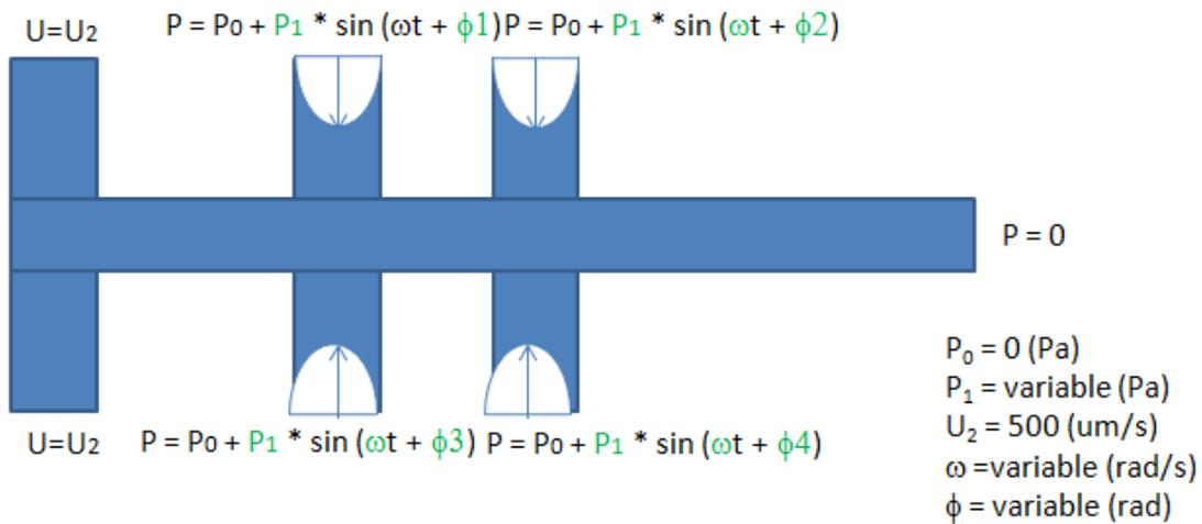
Figure 42: Navier-Stokes boundary conditions
