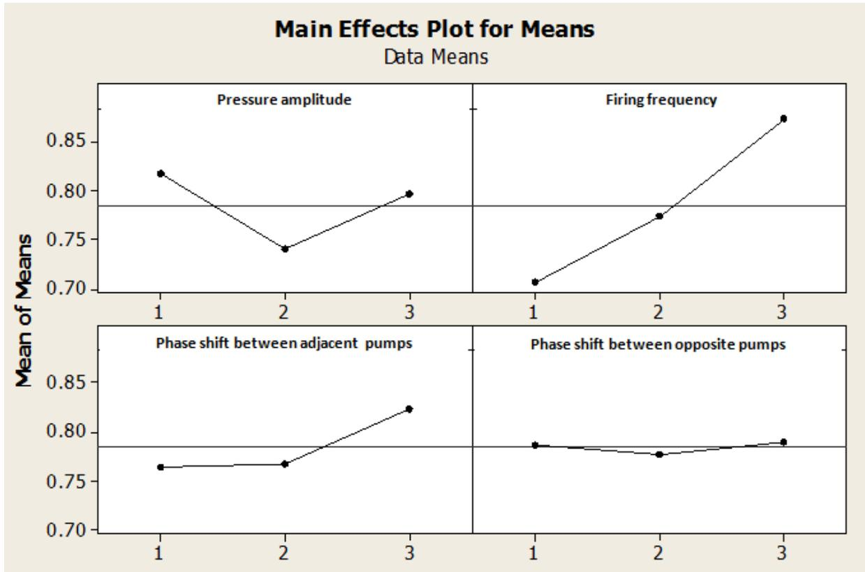
Figure 57: Mixing index dependence on design variables
