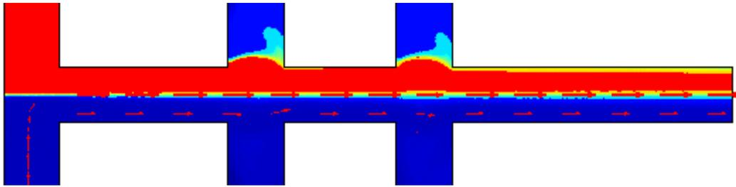
Figure 45: mixer solution at  $t=20\text{sec}$  for “normal” mesh
