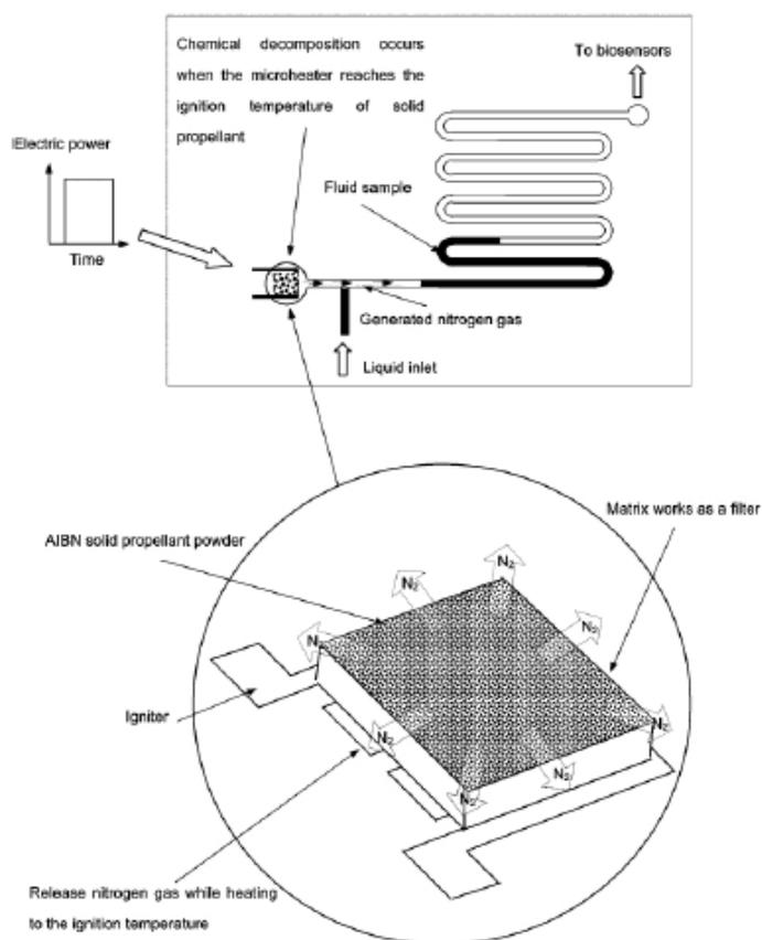
Figure 29: Schematic of AIBN-based micropump developed by Ahn<sub>28</sub>
