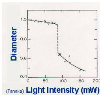
Figure 9: Light induced hydrogel phase transition
