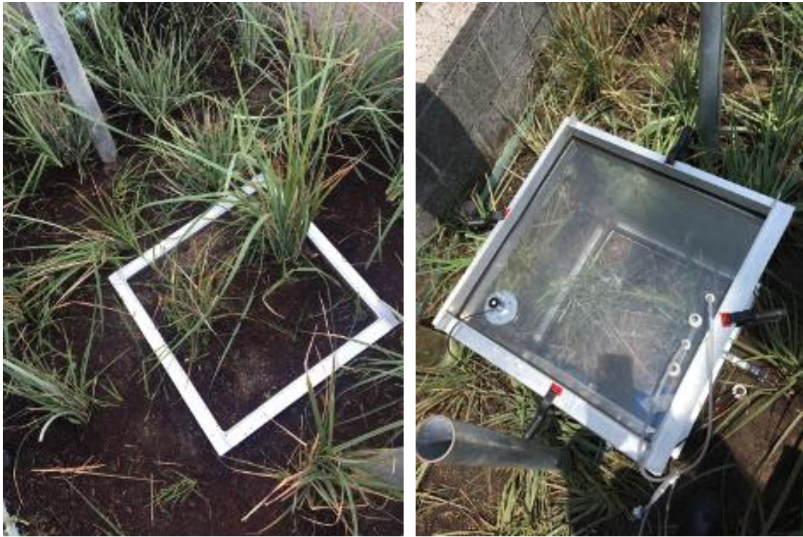
Figure S4. Chamber and metal base setup for CO 2 , CH 4 , and N 2 O sampling. The chamber was shaded with reflective material prior to gas flux measurements, which were taken for 2 to 3 minutes for CO 2 and CH 4 , and over a 30-minute period for N 2 O. Due to chamber shading, CO 2 emissions corresponded to ecosystem respiration since photosynthetic activity was excluded.
