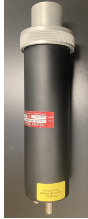
Figure 6.3: Scionix 38A38/2M-E1-BAF-X-NEG BaF 2 detector. The crystal is contained within the gray aluminum housing.
