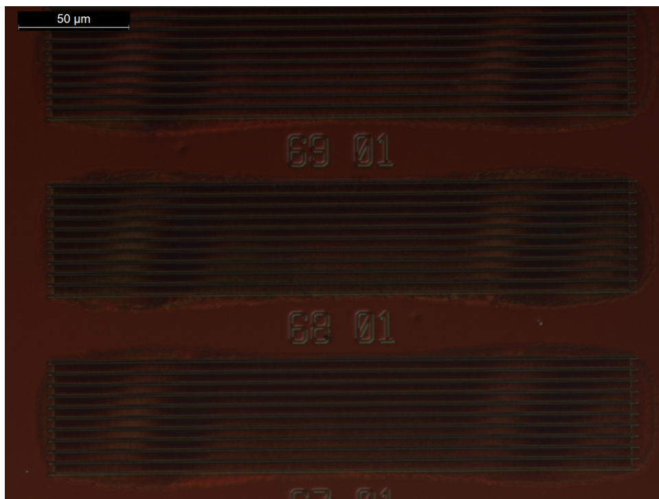
Figure A.5. Differential interference contrast image of PDMS film on SNM following backside etching with buffered oxide etch.
