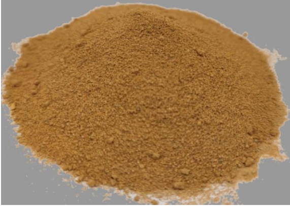
Figure 6.3. Tailings silty sand used in this study: (a) Collected sample, and (b) Grain size distribution.
