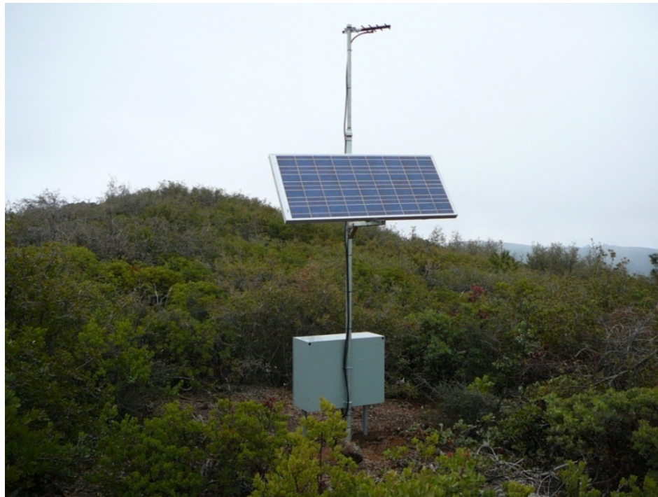
Figure 4-3. Radio Transmission Equipment and Solar Panel at a Typical Seismic Station
