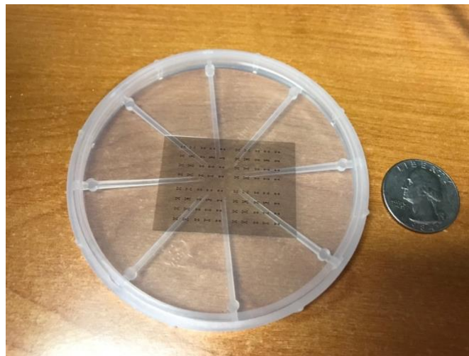
Figure 1-11: Final chip after whole fabrication process. Each pattern on the chip represents one surface acoustic wave delay line. The size comparison proves that acoustic wave devices have much smaller device size than electromagnetic wave devices.
