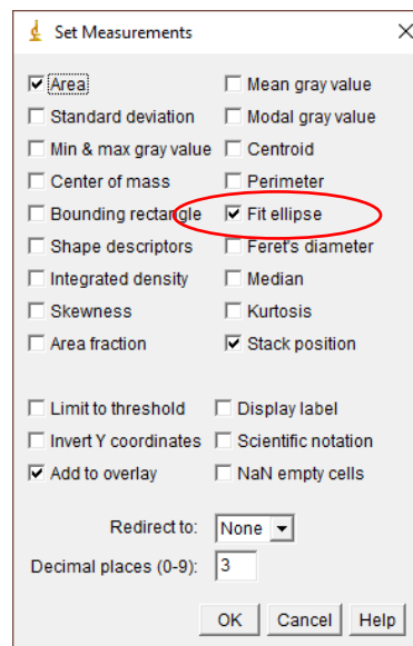
Figure G4 Check [Fit ellipse] to report Major and Minor lengths for particles.
