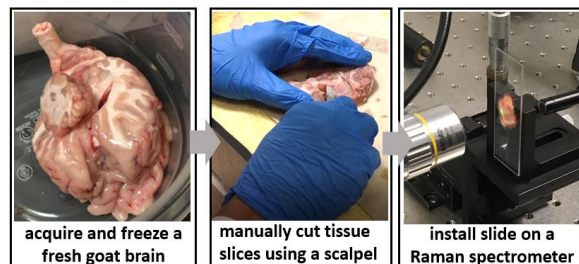
Figure 3 Preparation of tissue samples and installation on an open-bench Raman spectrometer.
