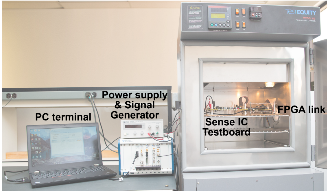
Figure 3.9: Temperature test for front-end linearity performance.
