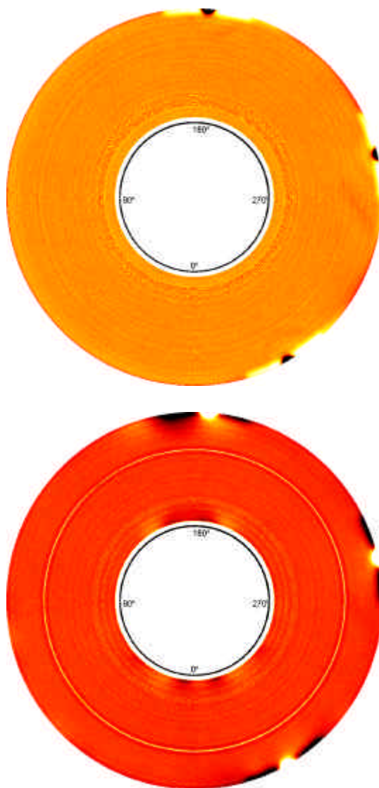
Figure 6.9 Images of disk after completion of experiment, obtained with optical surface analyzer (image on top is view of P-specula, image on bottom is view of Q-phase)
