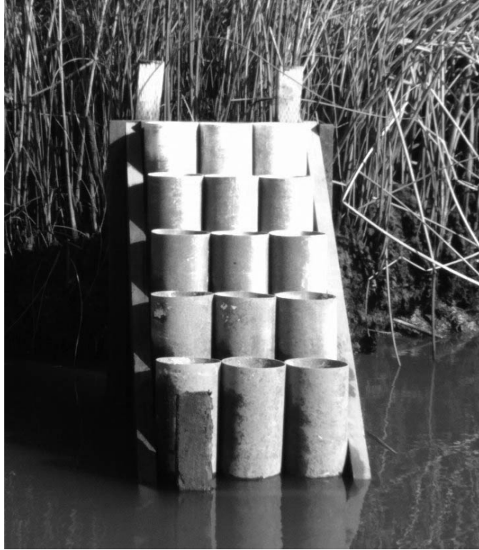
FIGURE 2-2. Example of an installed marsh organ before sediment and plants were added.
