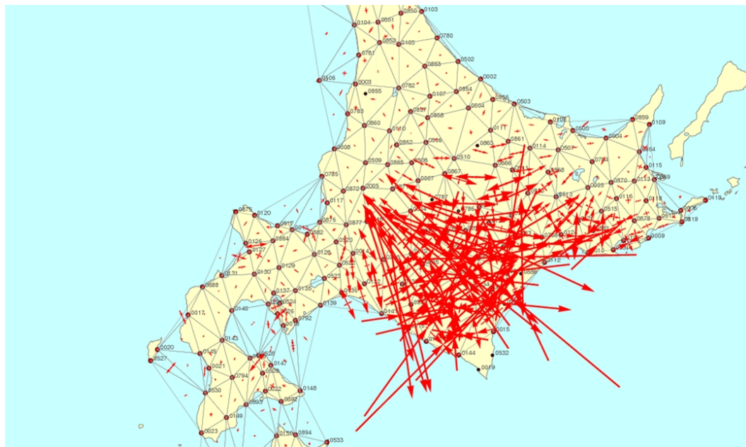
Figure 2.5: Delaunay triangulation of GEONET stations on Hokkaido Island and the two principal components of strain in each triangle one minute after the 2003 Mw 8.3 Tokachi-oki earthquake. From Crowell et al. [2009].
