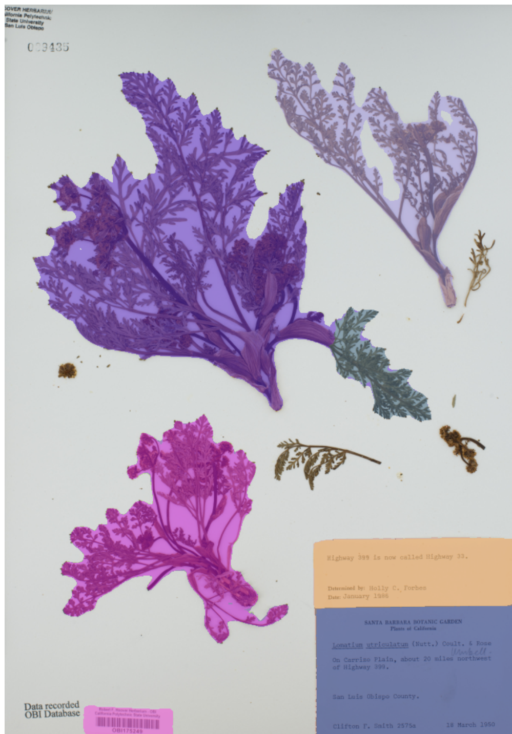
Figure 5.4: The output of the segmentation algorithm with masks overlaid on top of the segmented elements of interest. The label, barcode, herbarium stamp, and preserved plant are each isolated with clean boundaries and can be extracted for downstream processing. The segmentation of the label enables more structured and accurate downstream optical character recognition and natural language processing, and the segmentation of the plant specimen enables automated annotation of flowering status.
