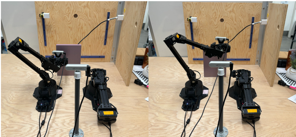
Figure 54: Spiral search initiated from the DLO connector's last known position (left) and workspace origin (right)
