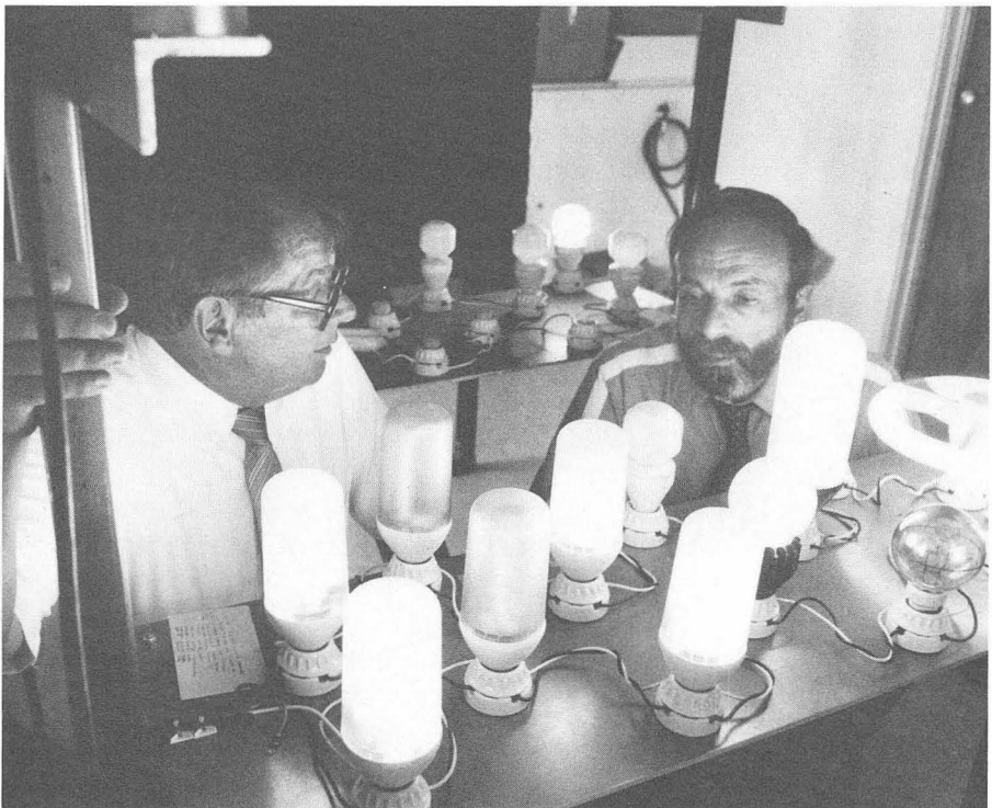
Examples of energy-efficient lamps. Visual and electrical properties are evaluated in LBL's Physical Lighting Laboratory.
