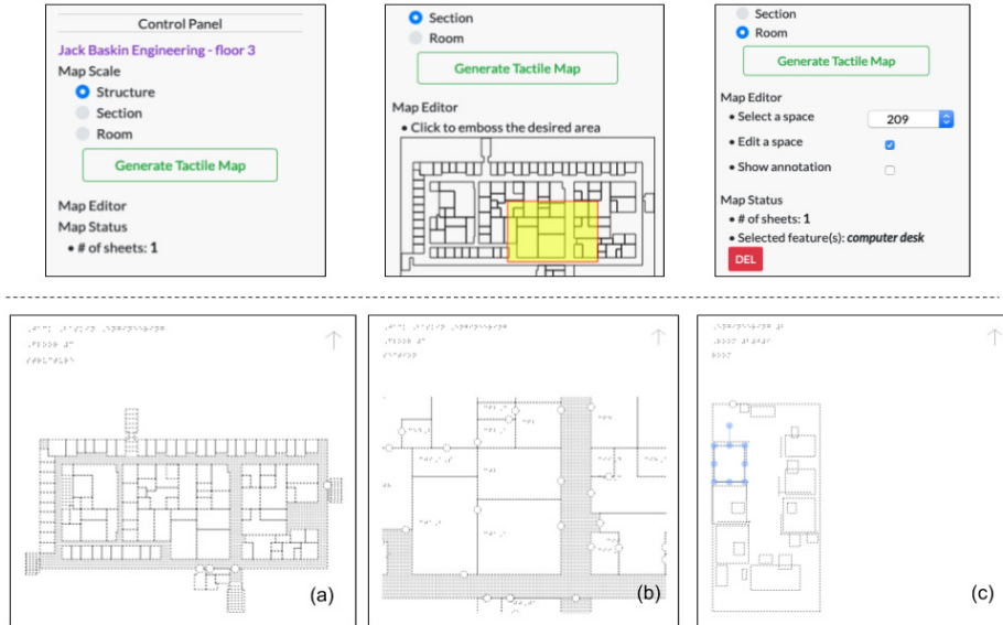
Fig. 2: The top row shows the M-EMAT control panels. The bottom row shows the generated tactile maps at 3 different scales: (a) structure, (b) section, and (c) room.
